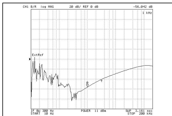
FIGURE 2-14: PSRR2-VPP (VPP = 225V + 1V AC).
