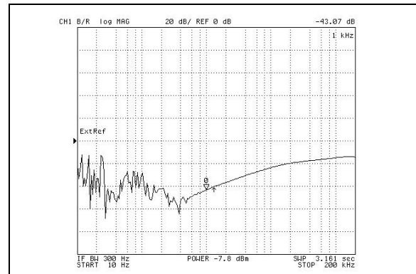
FIGURE 2-15: PSRR1-VDD (VDD = 5.0V + 0.1 V AC).
