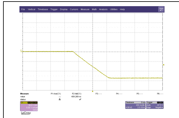
FIGURE 1-8: Typical HV_{OUT} from 0V to -135V, Load = 100pF
