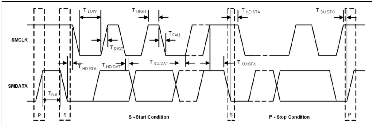
**FIGURE 4-1:** SMBus Timing Diagram.
