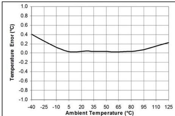
**FIGURE 2-3:** Temperature Error vs. Ambient Temperature (2N3904,  $T_{DIODE} = 42.5^\circ\text{C}$ ,  $V_{DD} = 3.3\text{V}$ ).
