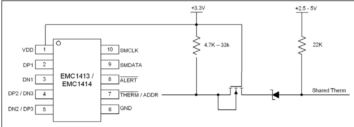
**FIGURE 4-2:** Isolating the THERM Pin.
