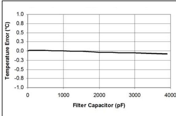
**FIGURE 2-1:** Temperature Error vs. Filter Capacitor (2N3904,  $T_A = 27^\circ\text{C}$ ,  $V_{DD} = 3.3\text{V}$ ).
