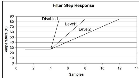
**FIGURE 5-3:** Temperature Filter Step Response.
