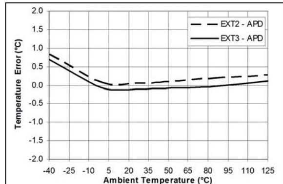
**FIGURE 2-6:** Temperature Error vs. Ambient Temperature (2N3904,  $T_A = 27^\circ\text{C}$ ,  $V_{DD} = 3.3\text{V}$ ).
