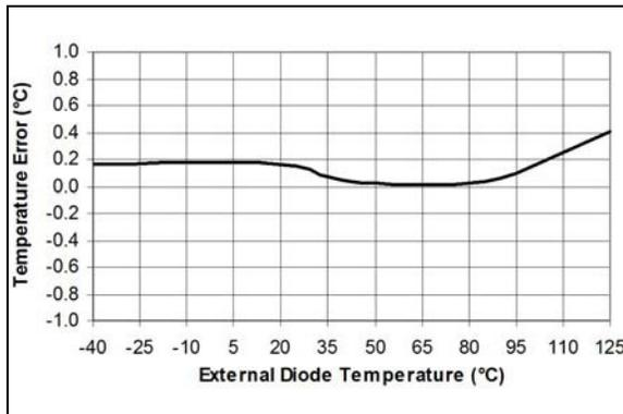
**FIGURE 2-2:** Temperature Error vs. External Diode Temperature (2N3904,  $T_A = 42.5^\circ\text{C}$ ,  $V_{DD} = 3.3\text{V}$ ).
