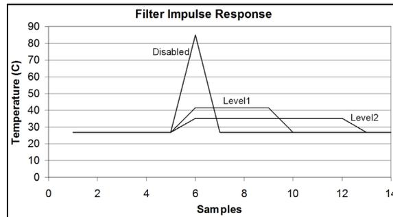
**FIGURE 5-4:** Temperature Filter Impulse Response.
