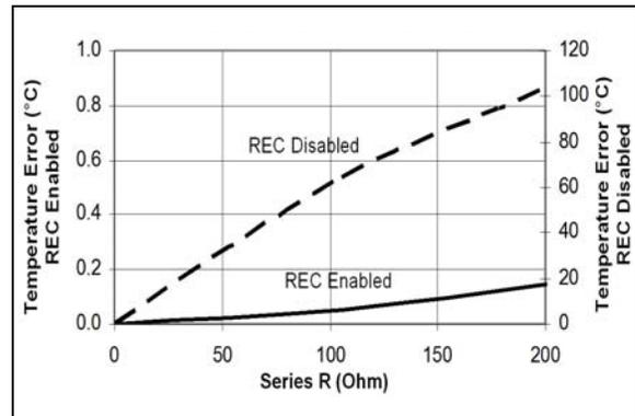
**FIGURE 2-5:** Temperature Error vs. Series Resistance.
