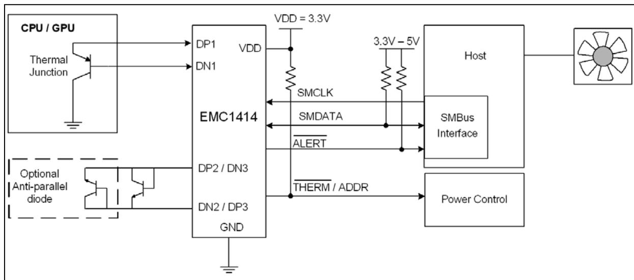
**FIGURE 5-1:** System Diagram for the EMC1414.
