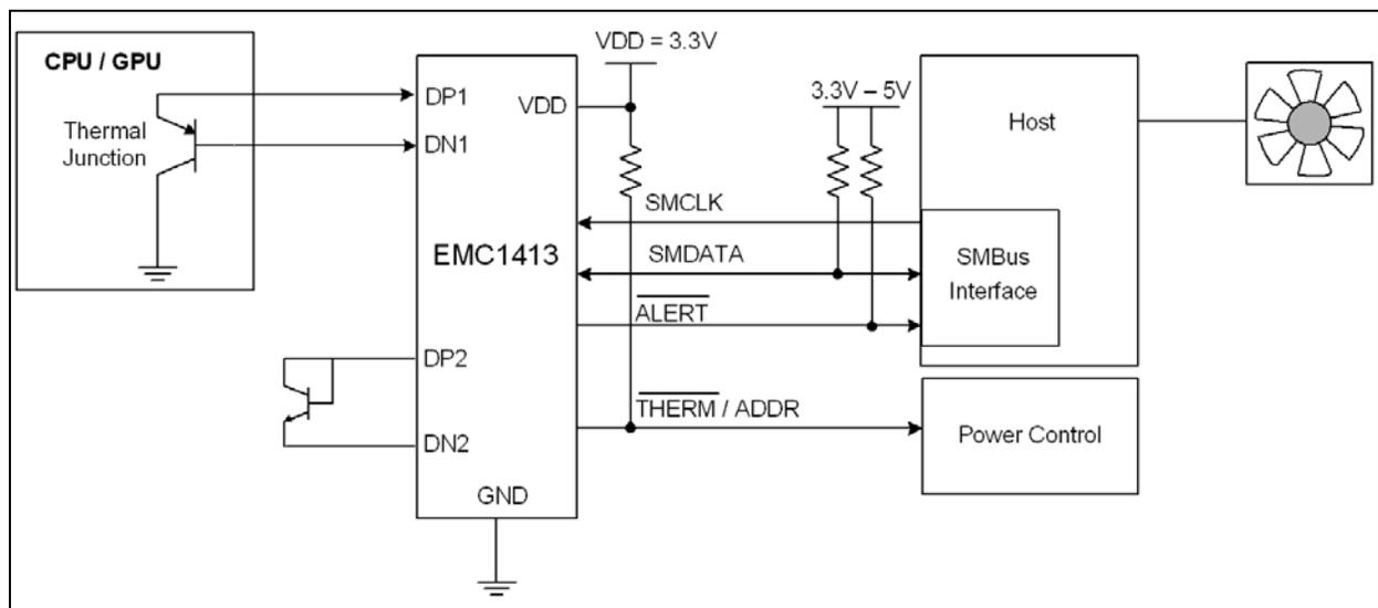
**FIGURE 5-2:** System Diagram for the EMC1413.
