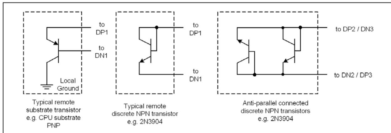
**FIGURE 5-5:** Diode Configurations for External Diode Channels.
