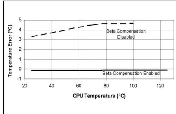
**FIGURE 2-4:** Temperature Error vs. CPU Temperature; Typical 65 nm CPU from Major Vendor ( $T_A = 27^\circ\text{C}$ ,  $V_{DD} = 3.3\text{V}$ ,  $BETA = 011$ ,  $C_{FILTER} = 470\text{ pF}$ ).
