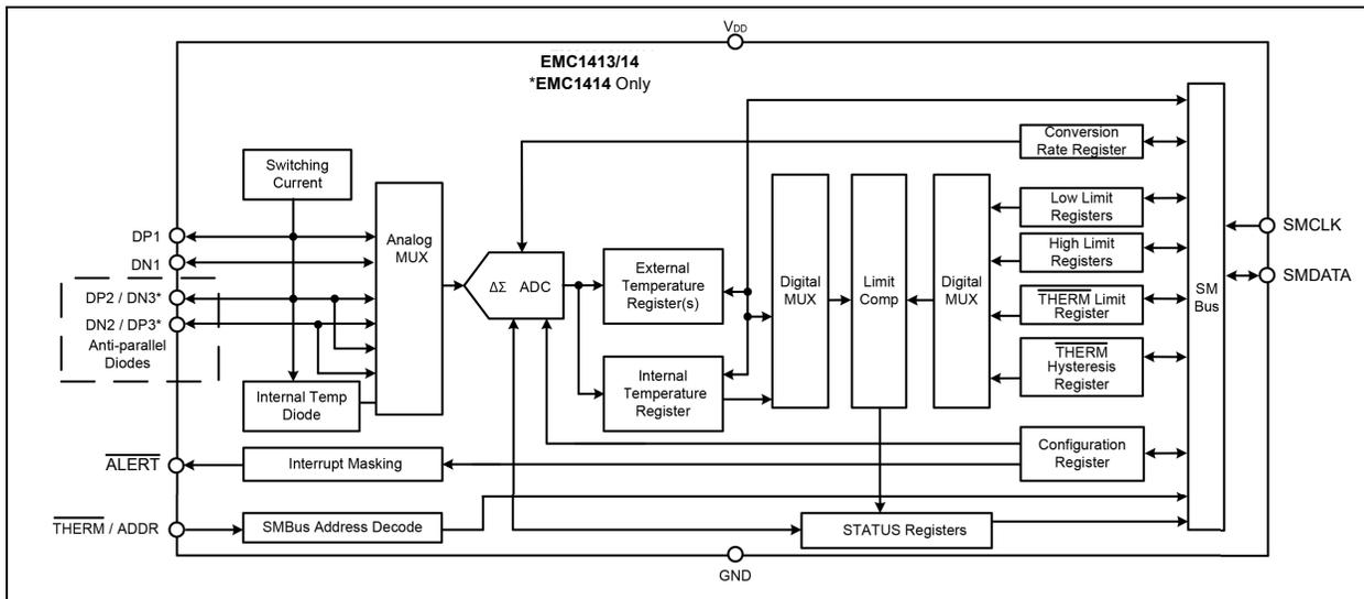
FIGURE 1: EMC1413/14 Block Diagram.
