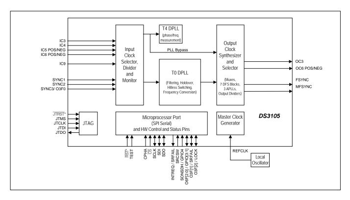
See Figure 7-1 for a detailed view of the T0 and T4 DPLLs and the Output Clock Synthesizer and Selector block.
