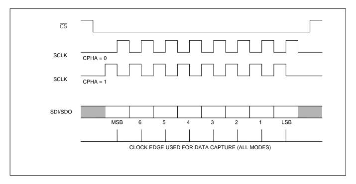
Figure 7-5. SPI Bus Transactions
