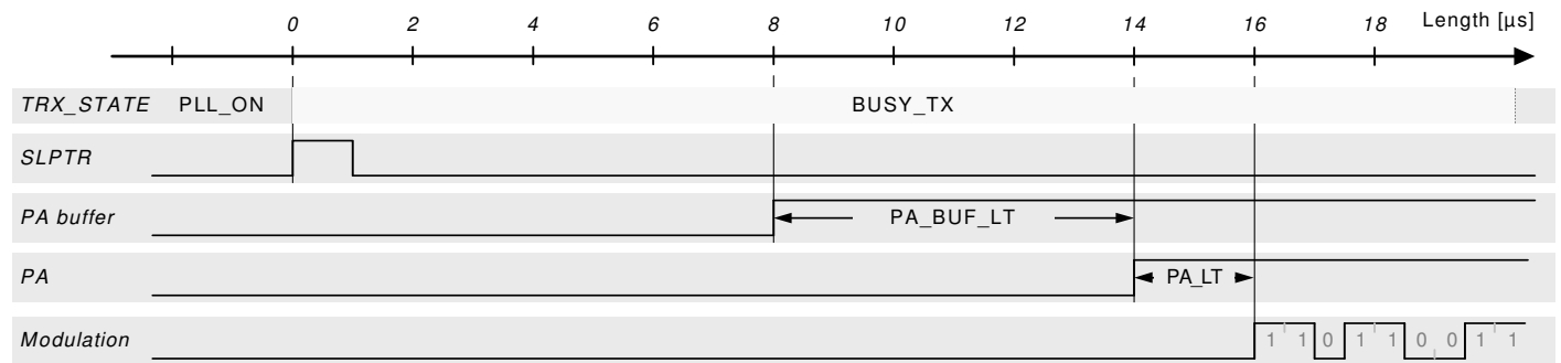
Figure 9-22. TX Power Ramping
