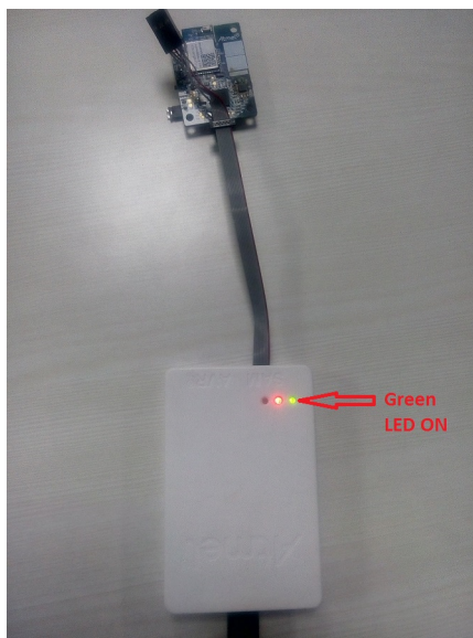
Figure 3-4. Atmel-ICE 10-pin Header Orientation
