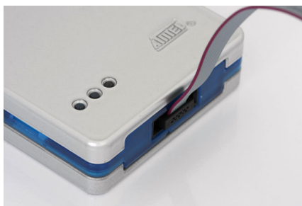
Figure 2-4. Atmel JTAGICE3 Cable Connection
