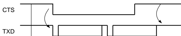
Figure 29-18. Transmitter Behavior when Operating with Hardware Handshaking
