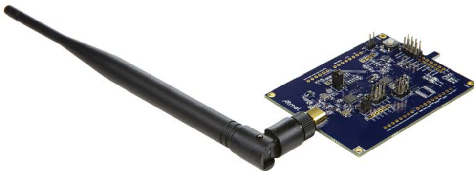
Figure 2-1. ATA8520-EK2-E Xplained Mini Extension Board with Attached External Antenna
