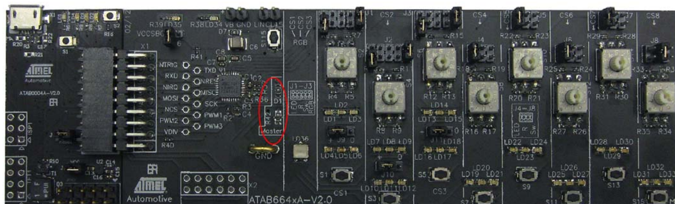
Figure 3-15. The Diode and Resistor Required for LIN Master Applications
