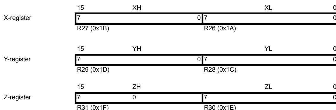
Figure 2-3. The X-, Y-, and Z-registers
