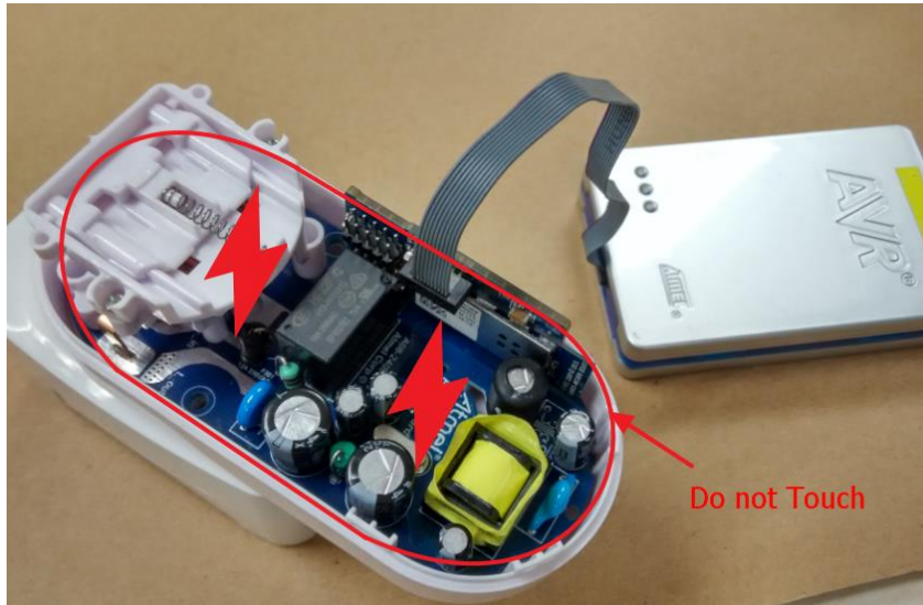
Figure 6-3. Kit Powered by the Onboard AC Input
