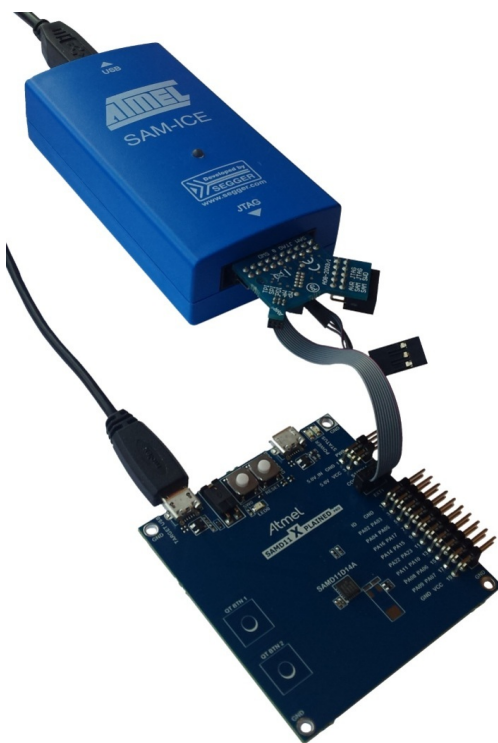
Figure 5-7. SAM-ICE using an Atmel-ICE Adapter
