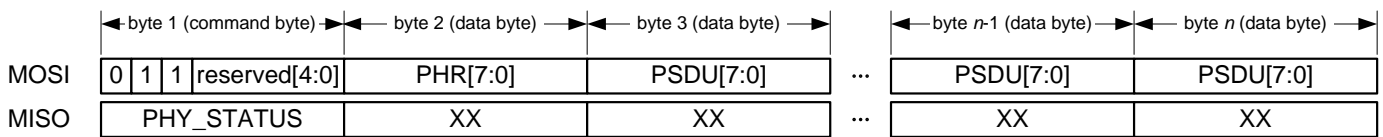
Figure 6-8. Packet Structure - Frame Write Access.
