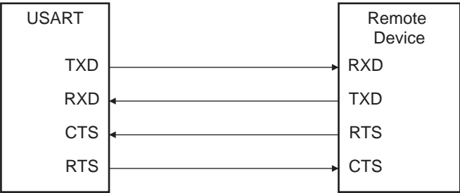
Figure 38-26. Connection with a Remote Device for Hardware Handshaking
