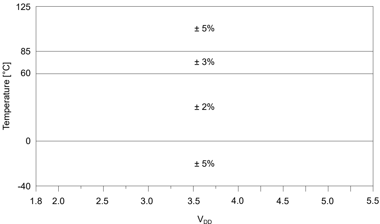
Figure 37-2. Precision Calibrated OSCHF (4 MHz) Frequency Accuracy Over Device V_{DD} and Temperature
