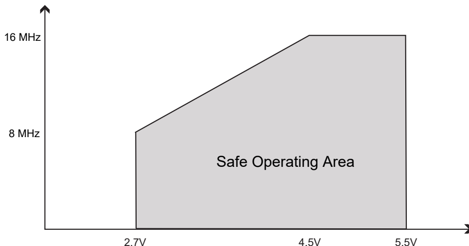
Figure 33-2. Maximum Frequency vs. V_{DD} for [85, 125]^{\circ}\text{C}
