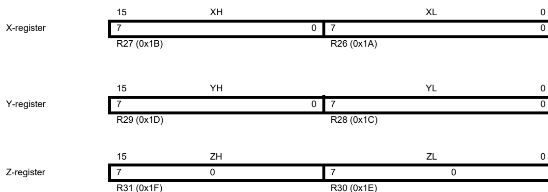
Figure 7-3. The X-, Y- and Z-Registers
