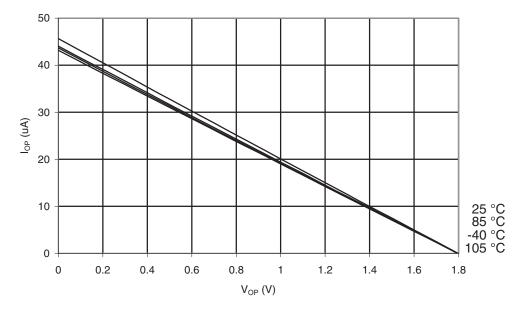
Figure 31-89. I/O Pin Pull-up Resistor Current vs. Input Voltage (V<sub>CC</sub> = 1.8V)
