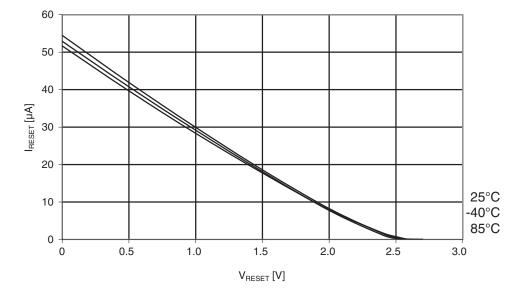
Figure 30-363. ATmega1284P: Reset pull-up resistor current vs. reset pin voltage (V<sub>cc</sub> = 2.7V)
