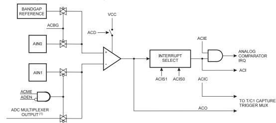
Figure 22-1. Analog Comparator block diagram (2)
