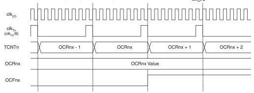
Figure 15-11 shows the setting of OCF0A and the clearing of TCNT0 in CTC mode and fast PWM mode where OCR0A is TOP.
