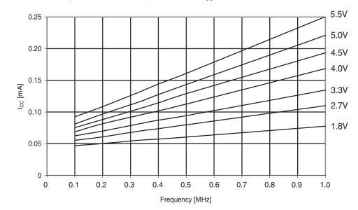
Figure 30-153. ATmega324PA: Idle supply current vs.  $V_{CC}$  (0.1 - 1.0MHz)
