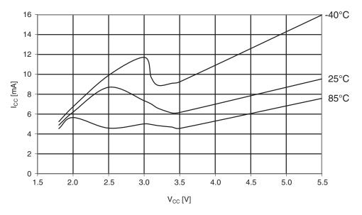
Figure 30-291. ATmega644PA: Watchdog timer current vs. V<sub>CC</sub>
