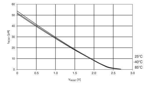
Figure 30-117. ATmega324A: Reset pull-up resistor current vs. reset pin voltage (V<sub>cc</sub> = 2.7V)
