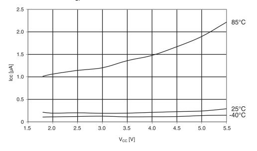
Figure 30-258. ATmega644PA: Power-save supply current vs. V<sub>CC</sub> (watchdog timer disabled and 32kHz crystal oscillator running)
