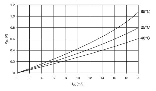
Figure 30-315. ATmega1284: I/O pin output voltage vs. sink current (V<sub>cc</sub> = 2.7V)
