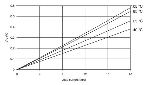
Figure 31-58. I/O Pin Output Voltage vs. Source Current (V<sub>cc</sub> = 3V)
