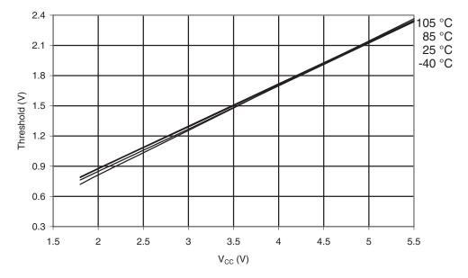
Figure 31-103. Reset Pin Input Threshold vs.  $V_{CC}$  (V<sub>IL</sub>, I/O Pin Read as '0')
