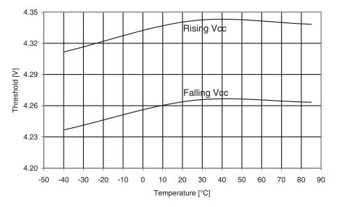
Figure 30-276. ATmega644PA: BOD threshold vs. temperature (V<sub>BOT</sub> = 4.3V)
