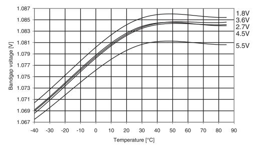
Figure 30-35. ATmega164A: Bandgap voltage vs. temperature.
