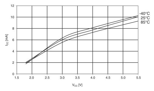
Figure 30-46. ATmega164A: Watchdog timer current vs. V<sub>cc</sub>
