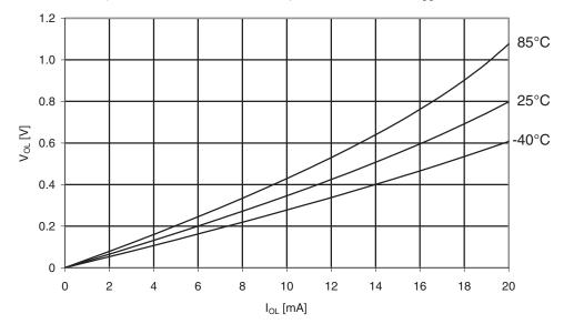
Figure 30-365. ATmega1284P: I/O pin output voltage vs. sink current (V<sub>cc</sub> = 2.7V)
