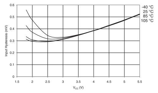
Figure 31-102. Reset Pin Input Threshold vs.  $V_{CC}$  (V $_{\rm IH}$  , I/O Pin Read as '1')
