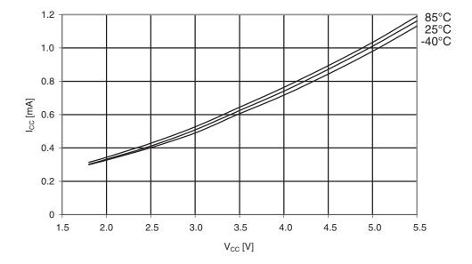
Figure 30-4. ATmega164A: Active supply current vs. V<sub>cc</sub> (internal RC oscillator, 1MHz)
