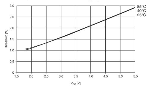
Figure 30-221. ATmega644A: I/O pin input threshold vs. V<sub>CC</sub> (V<sub>IH</sub> , I/O pin read as '1')
