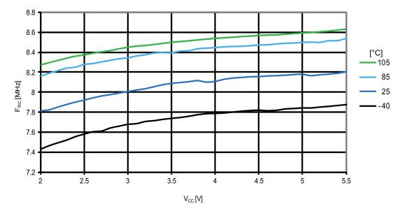
Figure 31-153. ATmega1284P: Calibrated 8MHz RC oscillator vs. V<sub>cc</sub>
