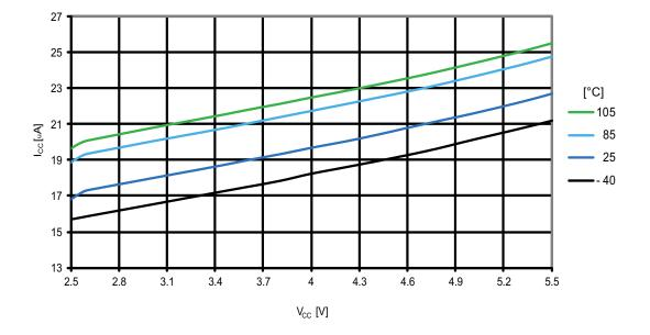
Figure 31-159. ATmega1284P: Brownout detector current vs. V<sub>cc</sub>
