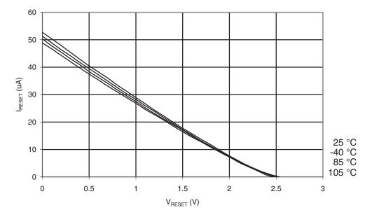
Figure 31-93. Reset Pull-up Resistor Current vs. Reset Pin Voltage (V<sub>CC</sub> = 2.7V)
