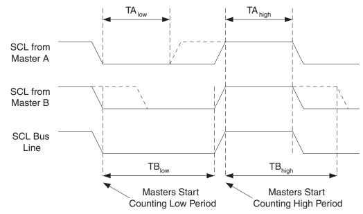
Figure 21-7. SCL synchronization between multiple masters
