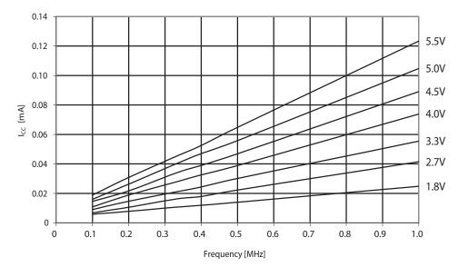
Figure 30-145. ATmega324A: Reset supply current vs. low frequency (0.1 - 1.0MHz)
