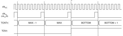
Figure 15-10 shows the setting of OCF0B in all modes and OCF0A in all modes except CTC mode and PWM mode, where OCR0A is TOP.
