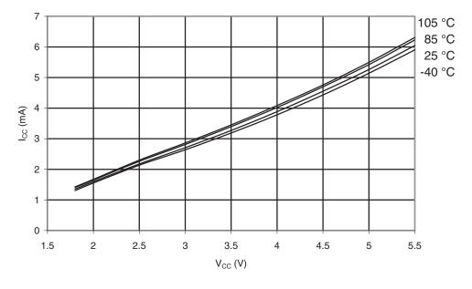
Figure 31-81. Active Supply Current vs. V<sub>cc</sub> (Internal RC Oscillator, 8 MHz)
