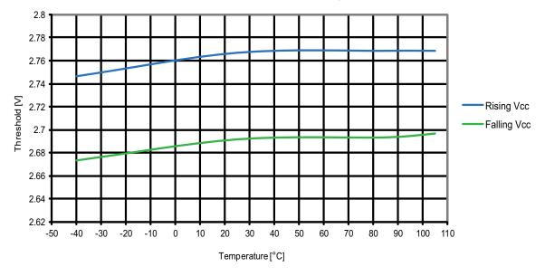
Figure 31-147. ATmega1284P: BOD threshold vs. temperature (V<sub>BOT</sub> = 2.7V)
