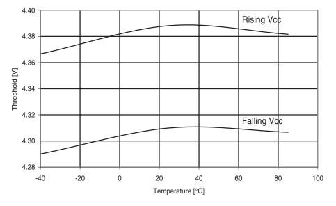
Figure 30-178. ATmega324PA: BOD threshold vs. temperature (V<sub>BOT</sub> = 4.3V).
