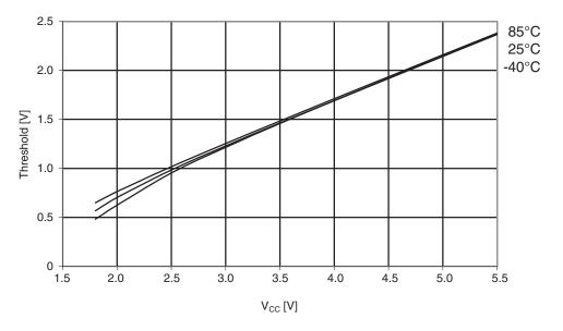
Figure 30-27. ATmega164A: I/O pin input hysteresis vs. V<sub>CC</sub>
