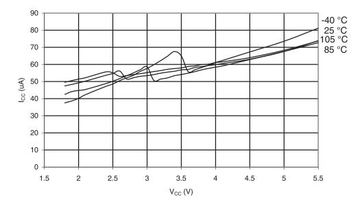
Figure 31-76. AREF External Reference Current vs. V<sub>cc</sub>
