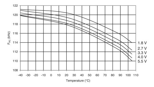
Figure 31-69. Watchdog Oscillator Frequency vs. Temperature
