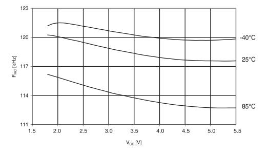
Figure 30-136. ATmega324A: Calibrated 8MHz RC oscillator vs.  $\rm V_{\rm CC}$
