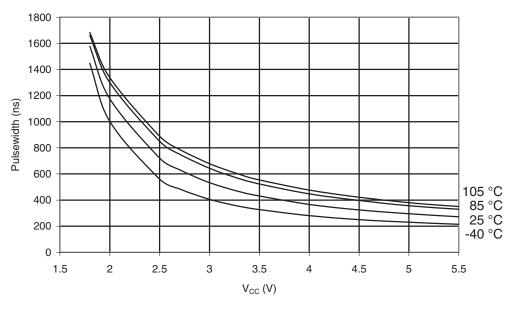
Figure 31-119. Minimum Reset Pulsewidth vs. Vcc
