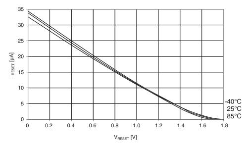
Figure 30-309. ATmega1284: I/O pin pull-up resistor current vs. input voltage (V<sub>CC</sub> = 1.8V)
