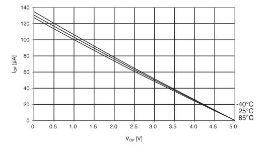
Figure 30-311. ATmega1284: I/O pin pull-up resistor current vs. input voltage (V<sub>cc</sub> = 5V)
