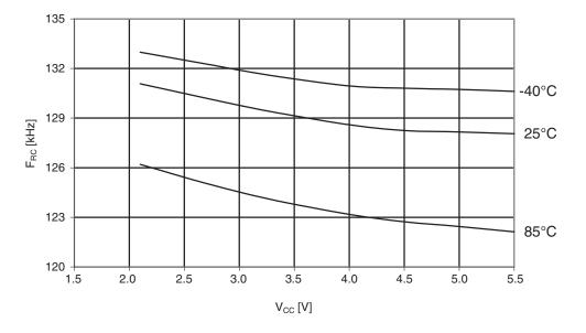
Figure 30-87. ATmega164PA: Calibrated 8MHz RC oscillator vs. V<sub>cc</sub>
