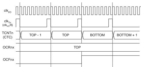
Figure 17-11. Timer/Counter Timing diagram, Clear Timer on Compare Match mode, with prescaler (f<sub>clk I/O</sub>/8)
