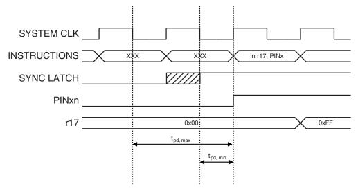
Consider the clock period starting shortly after the first falling edge of the system clock. The latch is closed when the clock is low, and goes transparent when the clock is high, as indicated by the shaded region of the "SYNC LATCH" signal. The signal value is latched when the system clock goes low. It is clocked into the PINxn Register at the succeeding positive clock edge. As indicated by the two arrows tpd,max and tpd,min, a single
