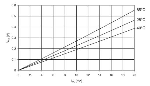
Figure 30-317. ATmega1284: I/O pin output voltage vs. sink current (V<sub>cc</sub> = 5V)
