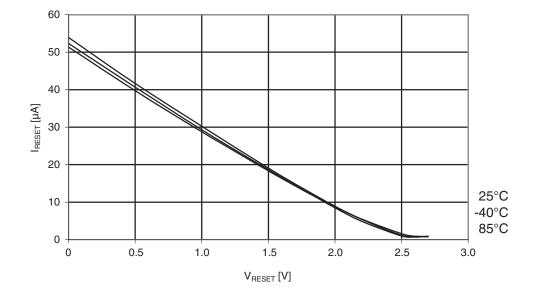
Figure 30-68. ATmega164PA: Reset pull-up resistor current vs. reset pin voltage (V<sub>cc</sub> = 2.7V)
