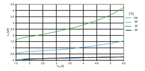
Figure 31-7. ATmega164PA: Power-down supply current vs. V<sub>CC</sub> (watchdog timer disabled)
