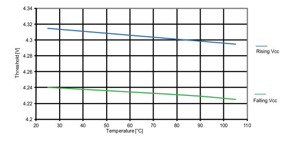
Figure 31-25. ATmega164PA: BOD threshold vs. temperature (V<sub>BOT</sub> = 4.3V)
