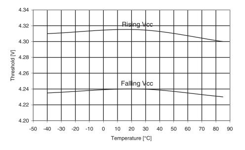
Figure 30-31. ATmega164A: BOD threshold vs. temperature (V<sub>BOT</sub> = 4.3V)
