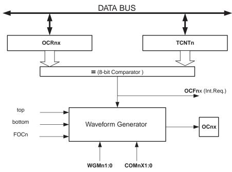
Figure 15-3. Output Compare unit, block diagram
