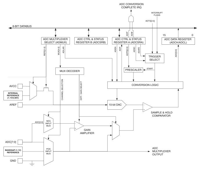
Figure 23-1. Analog-to-digital Converter block schematic
