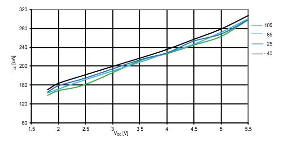
Figure 31-35. ATmega164PA: ADC current vs.  $V_{cc}$  (AREF =  $AV_{cc}$ )
