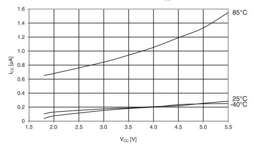
Figure 30-11. ATmega164A: Power-down supply current vs. V<sub>cc</sub> (watchdog timer disabled)
