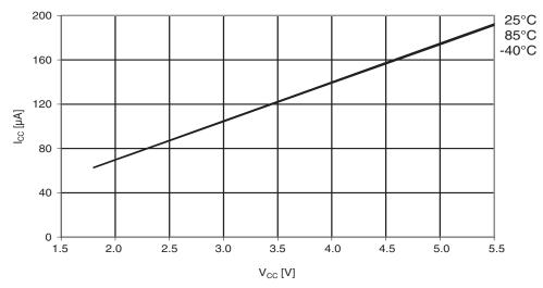
Figure 30-92. ATmega164PA: AREF external reference current vs. V<sub>cc</sub>
