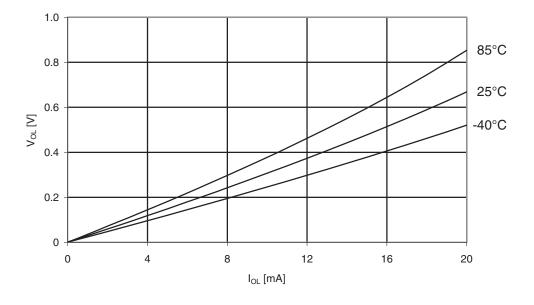
Figure 30-21. ATmega164A: I/O pin output voltage vs. sink current (V<sub>CC</sub> = 3V)
