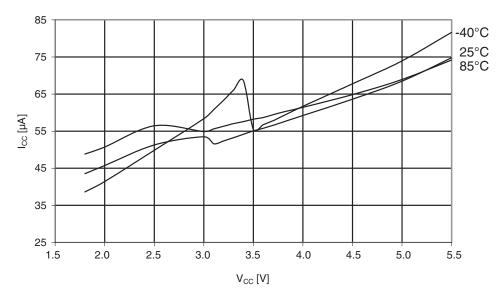
Figure 30-388. ATmega1284P: AREF external reference current vs. V<sub>CC</sub>
