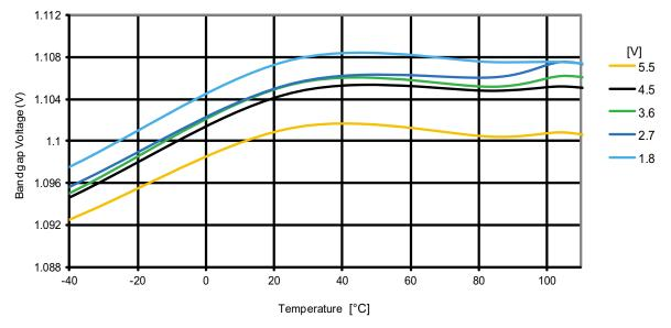
Figure 31-29. ATmega164PA: Bandgap voltage vs. temperature
