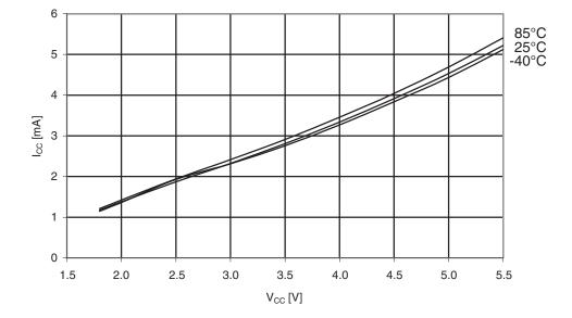
Figure 30-52. ATmega164PA: Active supply current vs. V<sub>CC</sub> (internal RC oscillator, 8MHz)
