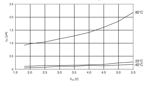
Figure 30-256. ATmega644PA: Power-down supply current vs. V<sub>CC</sub> (watchdog timer disabled)
