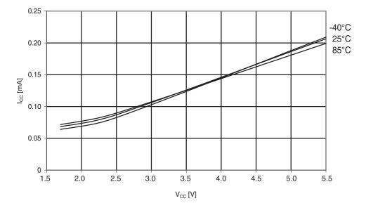
Figure 30-103. ATmega324A: Active supply current vs. V<sub>CC</sub> (internal RC oscillator, 128kHz)
