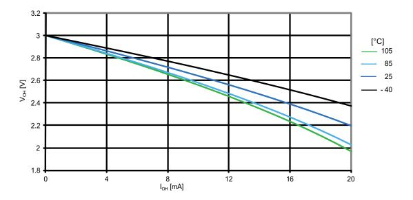
Figure 31-17. ATmega164PA: I/O pin output voltage vs. source current (V<sub>cc</sub> = 3V)
