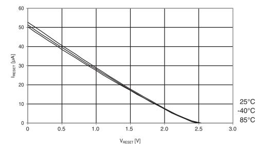
Figure 30-216. ATmega644A: Reset pull-up resistor current vs. reset pin voltage (V<sub>cc</sub> = 5V)
