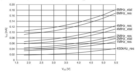
Figure 30-63. ATmega164PA: Standby supply current vs. V<sub>CC</sub> (watchdog timer disabled)
