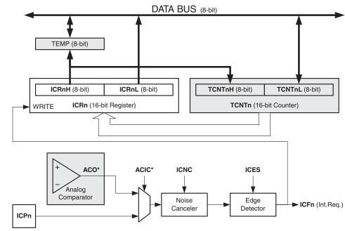
Figure 16-3. Input Capture unit block diagram
