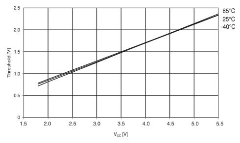
Figure 30-225. ATmega644A: Reset pin input threshold vs.  $V_{CC}$  ( $V_{IL}$ , I/O pin read as '0')
