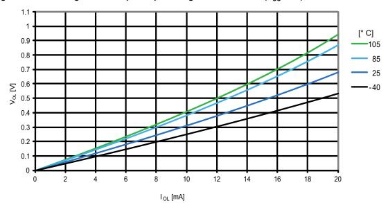
Figure 31-136. ATmega1284P: I/O pin output voltage vs. sink current (V<sub>cc</sub> = 3V)
