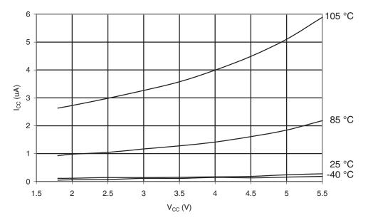
Figure 31-87. Power-down Supply Current vs. V<sub>CC</sub> (Watchdog Timer Disabled)
