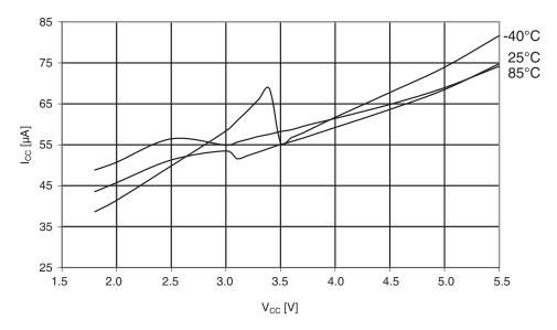
Figure 30-338. ATmega1284: AREF external reference current vs. V<sub>CC</sub>
