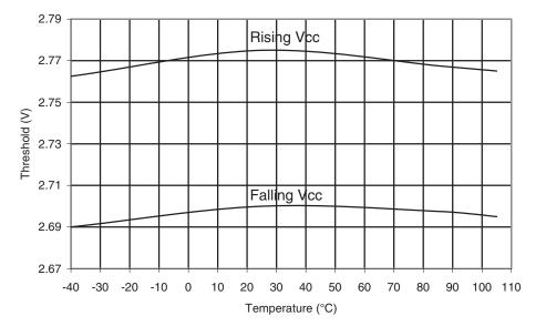
Figure 31-68. BOD Threshold vs. Temperature (V<sub>cc</sub> = 1.8V)
