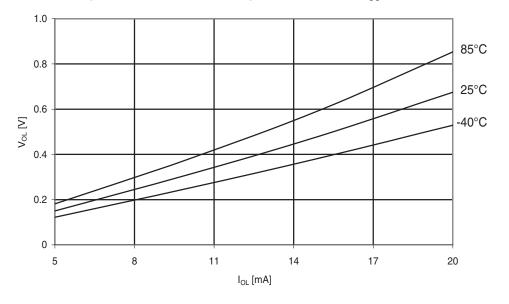
Figure 30-119. ATmega324A: I/O pin output voltage vs. sink current (V<sub>CC</sub> = 3V)
