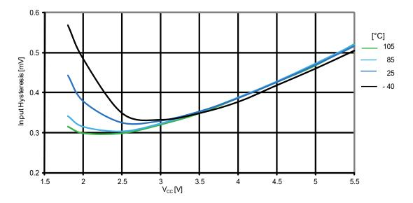
Figure 31-22. ATmega164PA: Reset pin input threshold vs. V<sub>CC</sub> (V<sub>IH</sub> , I/O pin read as '1')
