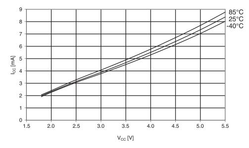
Figure 30-297. ATmega1284: Active supply current vs. V<sub>cc</sub> (internal RC oscillator, 8MHz)
