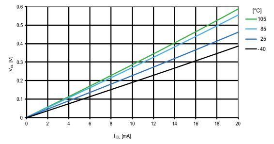
Figure 31-137. ATmega1284P: I/O pin output voltage vs. sink current (V<sub>cc</sub> = 5V)
