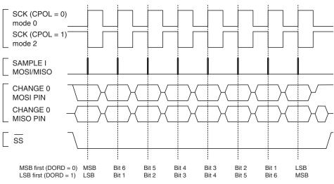
Figure 18-4. SPI transfer format with CPHA = 1
