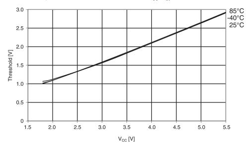
Figure 30-270. ATmega644PA: I/O pin input threshold vs. V<sub>CC</sub> (V<sub>IH</sub> , I/O pin read as '1')
