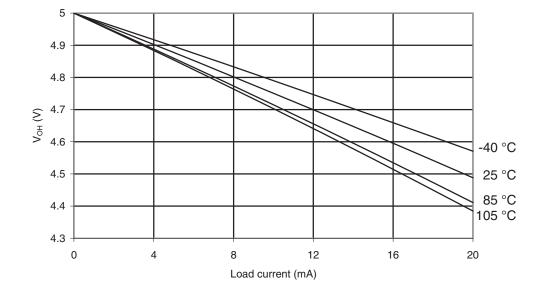
Figure 31-59. I/O Pin Output Voltage vs. Source Current (V<sub>cc</sub> = 5V)
