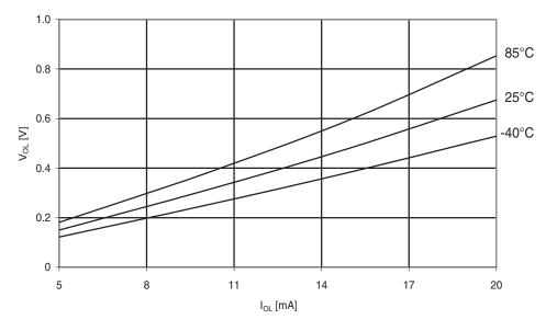
Figure 30-168. ATmega324PA: I/O pin output voltage vs. sink current (V<sub>cc</sub> = 3V)
