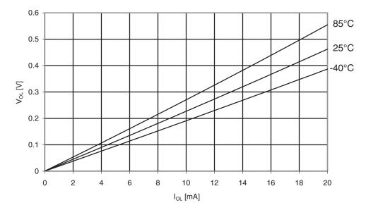
Figure 30-367. ATmega1284P: I/O pin output voltage vs. sink current (V<sub>cc</sub> = 5V)
