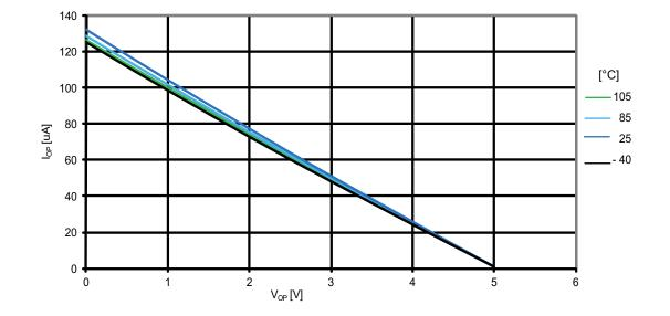
Figure 31-11. ATmega164PA: I/O pin pull-up resistor current vs. input voltage (V<sub>cc</sub> = 5V)
