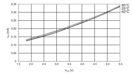
Figure 30-205. ATmega644A: Idle supply current vs. V<sub>CC</sub> (internal RC oscillator, 1MHz)
