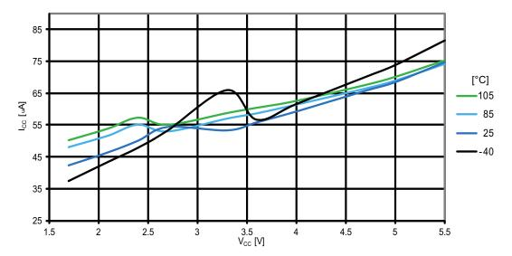
Figure 31-157. ATmega1284P: Analog comparator current vs. V<sub>cc</sub>
