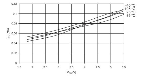
Figure 31-47. Idle Supply Current vs. V<sub>cc</sub> (Internal RC Oscillator, 128 kHz)
