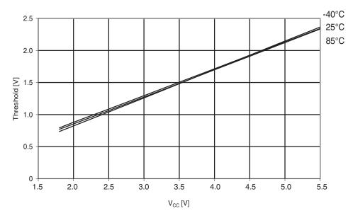
Figure 30-176. ATmega324PA: Reset pin input threshold vs. V<sub>CC</sub> (V<sub>IL</sub>, I/O pin read as '0')
