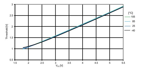
Figure 31-19. ATmega164PA: I/O pin input threshold vs. V<sub>CC</sub> (V<sub>IH</sub>, I/O pin read as '1')
