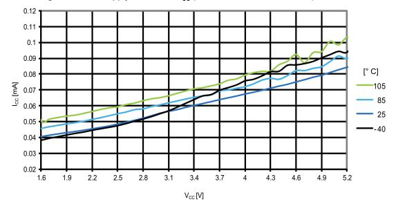
Figure 31-125. ATmega1284P: Idle supply current vs. V<sub>CC</sub> (internal RC oscillator, 128kHz)
