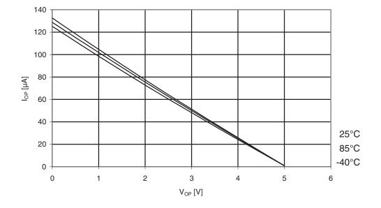
Figure 30-66. ATmega164PA: I/O pin pull-up resistor current vs. input voltage (V<sub>cc</sub> = 5V)
