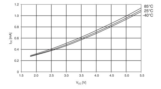
Figure 30-8. ATmega164A: Idle supply current vs. V<sub>CC</sub> (internal RC oscillator, 8MHz)
