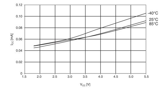
Figure 30-10. ATmega164A: Idle supply current vs. V<sub>cc</sub> (internal RC oscillator, 128kHz)
