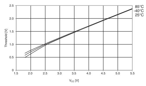
Figure 30-371. ATmega1284P: I/O pin input threshold vs.  $V_{CC}$  ( $V_{IL}$ , I/O pin read as '0')
