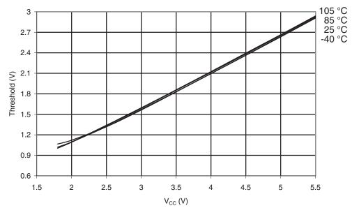
Figure 31-99. I/O Pin Input Threshold vs. V<sub>CC</sub> (V<sub>IH</sub>, I/O Pin Read as '1')
