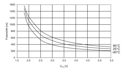
Figure 30-98. ATmega164PA: Minimum reset pulsewidth vs. V<sub>cc</sub>
