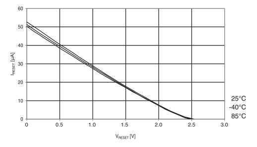
Figure 30-265. ATmega644PA: Reset pull-up resistor current vs. reset pin voltage (V<sub>cc</sub> = 5V)
