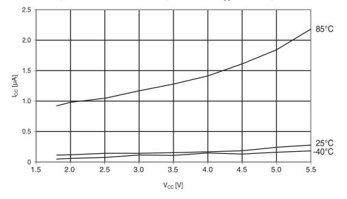
Figure 30-207. ATmega644A: Power-down supply current vs. V<sub>cc</sub> (watchdog timer disabled)
