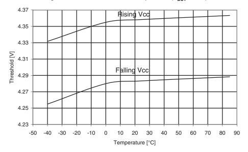
Figure 30-376. ATmega1284P: BOD threshold vs. temperature (V<sub>BOT</sub> = 4.3V)
