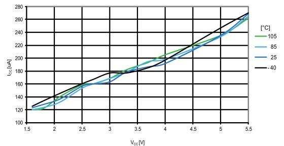
Figure 31-156. ATmega1284P: ADC current vs. V<sub>cc</sub> (AREF = AV<sub>cc</sub>)
