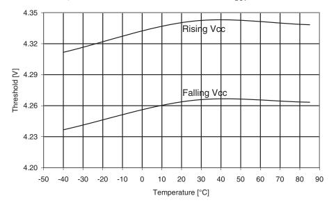
Figure 30-227. ATmega644A: BOD threshold vs. temperature (V<sub>BOT</sub> = 4.3V)
