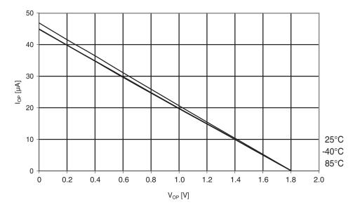
Figure 30-113. ATmega324A: I/O pin pull-up resistor current vs. input voltage (V<sub>cc</sub> = 1.8V)
