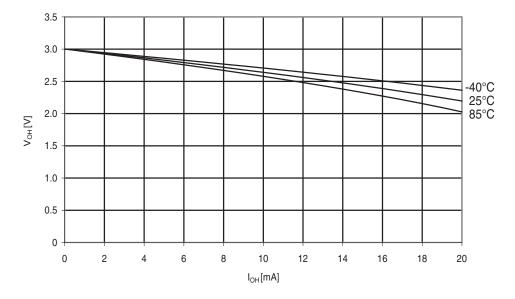
Figure 30-219. ATmega644A: I/O pin output voltage vs. source current (V<sub>cc</sub> = 3V)
