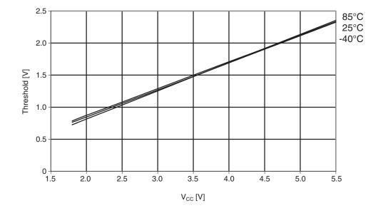
Figure 30-78. ATmega164PA: Reset pin input threshold vs. V<sub>CC</sub> (V<sub>IL</sub>, I/O pin read as '0')
