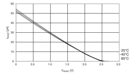
Figure 30-313. ATmega1284: Reset pull-up resistor current vs. reset pin voltage (V<sub>cc</sub> = 2.7V)
