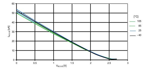
Figure 31-13. ATmega164PA: Reset pull-up resistor current vs. reset pin voltage ( $V_{cc}$  = 2.7V)
