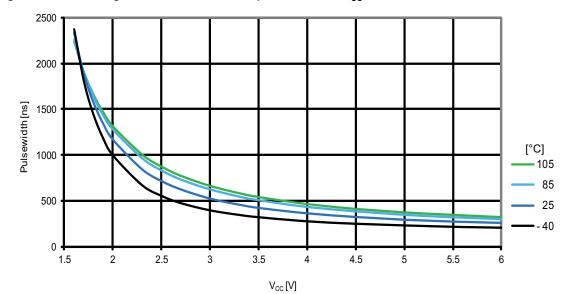
Figure 31-162. ATmega1284P: Minimum reset pulsewidth vs. V<sub>cc</sub>
