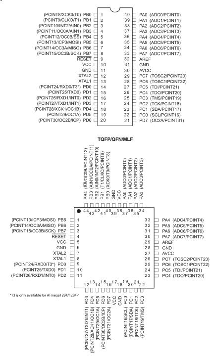
Note: The large center pad underneath the VQFN/QFN/MLF package should be soldered to ground on the board to ensure good mechanical stability.
