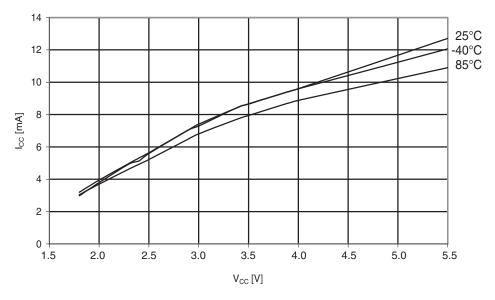
Figure 30-193. ATmega324PA: Watchdog timer current vs. V<sub>cc</sub>
