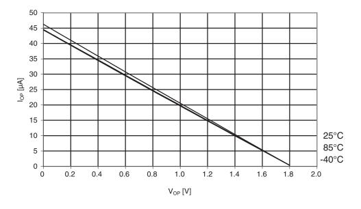
Figure 30-15. ATmega164A: I/O pin pull-up resistor current vs. Input voltage (V<sub>cc</sub> = 1.8V)
