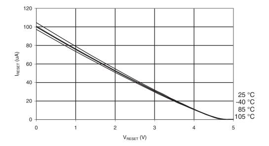
Figure 31-55. Reset Pull-up Resistor Current vs. Reset Pin Voltage (V<sub>cc</sub> = 5V)
