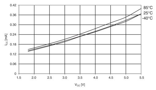
Figure 30-353. ATmega1284P: Idle supply current vs. V<sub>cc</sub> (internal RC oscillator, 1MHz)
