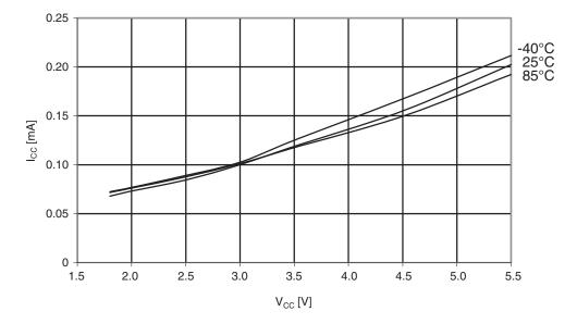
Figure 30-54. ATmega164PA: Active supply current vs. V<sub>cc</sub> (internal RC oscillator, 128kHz)
