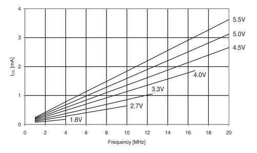
Figure 30-106. ATmega324A: Idle supply current vs. V<sub>cc</sub> (internal RC oscillator, 8MHz)
