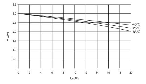
Figure 30-268. ATmega644PA: I/O pin output voltage vs. source current (V<sub>cc</sub> = 3V)
