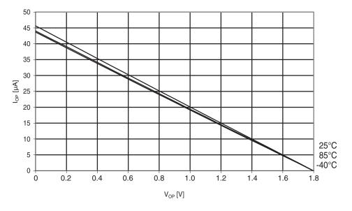
Figure 30-211. ATmega644A: I/O pin pull-up resistor current vs. input voltage (V<sub>cc</sub> = 1.8V)
