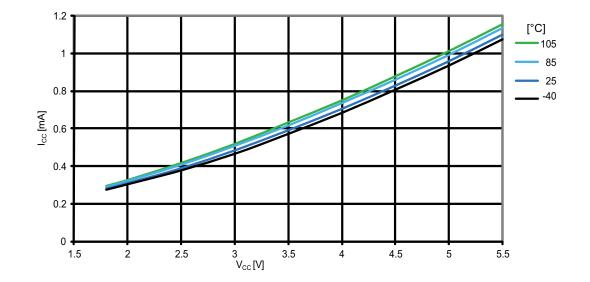
Figure 31-5. ATmega164PA: Idle supply current vs. V<sub>CC</sub> (internal RC oscillator, 1MHz)
