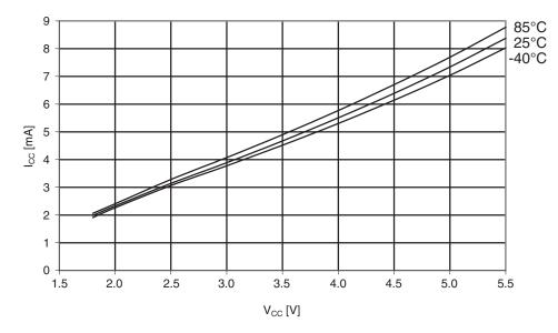
Figure 30-347. ATmega1284P: Active supply current vs. V<sub>CC</sub> (internal RC oscillator, 8MHz)
