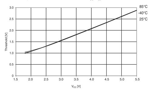
Figure 30-123. ATmega324A: I/O pin input threshold vs. V<sub>CC</sub> (V<sub>IH</sub> , I/O pin read as '1')
