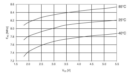
Figure 30-333. ATmega1284: Calibrated 8MHz RC oscillator vs. V<sub>cc</sub>
