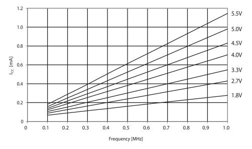
Figure 30-148. ATmega324PA: Active supply current vs. low frequency (0.1 - 1.0MHz)
