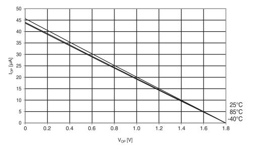
Figure 30-260. ATmega644PA: I/O pin pull-up resistor current vs. input voltage (V<sub>CC</sub> = 1.8V)
