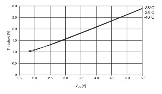
Figure 30-74. ATmega164PA: I/O pin input threshold vs. V<sub>CC</sub> (V<sub>IH</sub>, I/O pin read as '1')
