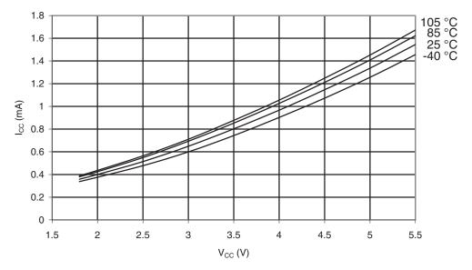
Figure 31-45. Idle Supply Current vs. V<sub>cc</sub> (Internal RC Oscillator, 8 MHz)
