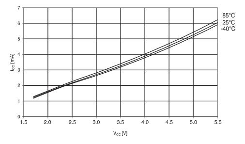
Figure 30-199. ATmega644A: Active supply current vs. V<sub>CC</sub> (internal RC oscillator, 8MHz)
