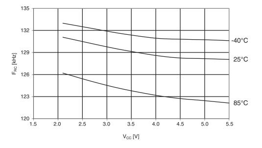
Figure 30-38. ATmega164A: Calibrated 8MHz RC oscillator vs.  $V_{\text{CC}}$
