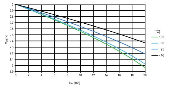
Figure 31-139. ATmega1284P: I/O pin output voltage vs. source current (V<sub>cc</sub> = 3V)
