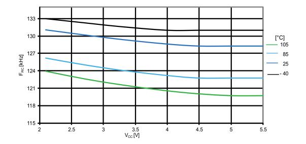
Figure 31-31. ATmega164PA: Watchdog oscillator frequency vs. V<sub>cc</sub>
