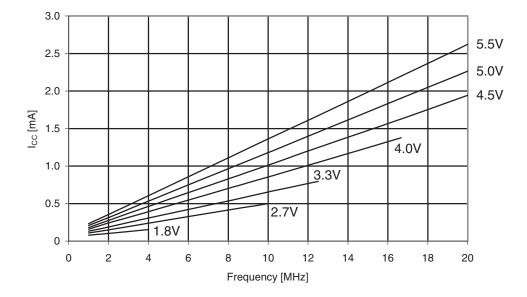
Figure 30-56. ATmega164PA: Idle supply current vs. V<sub>cc</sub> (1 - 20MHz)
