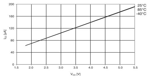
Figure 30-43. ATmega164A: AREF external reference current vs. V<sub>cc</sub>
