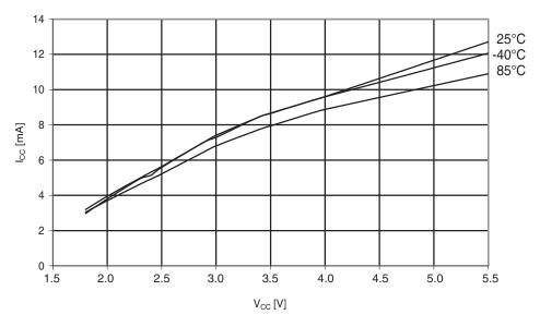
Figure 30-144. ATmega324A: Watchdog timer current vs. V<sub>cc</sub>
