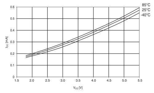
Figure 30-156. ATmega324PA: Idle supply current vs. V<sub>CC</sub> (internal RC oscillator, 1MHz)
