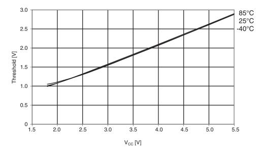
Figure 30-25. ATmega164A: I/O pin input threshold vs. V<sub>CC</sub> (V<sub>IH</sub> I/O pin read as '1')
