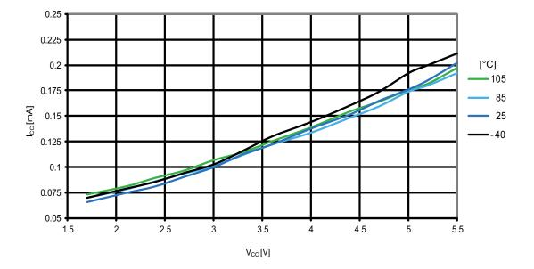
Figure 31-3. ATmega164PA: Active supply current vs. V<sub>CC</sub> (internal RC oscillator, 128kHz)
