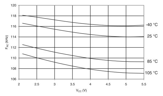
Figure 31-110. Calibrated 8 MHz RC Oscillator vs.  $V_{\text{CC}}$
