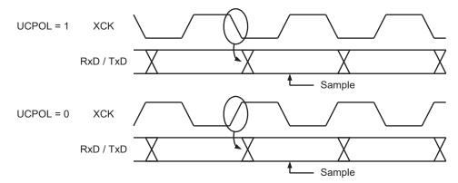
The UCPOLn bit UCRSC selects which XCKn clock edge is used for data sampling and which is used for data change. As Figure 19-3 on page 179 shows, when UCPOLn is zero the data will be changed at rising XCKn edge and sampled at falling XCKn edge. If UCPOLn is set, the data will be changed at falling XCKn edge and sampled at rising XCKn edge.
