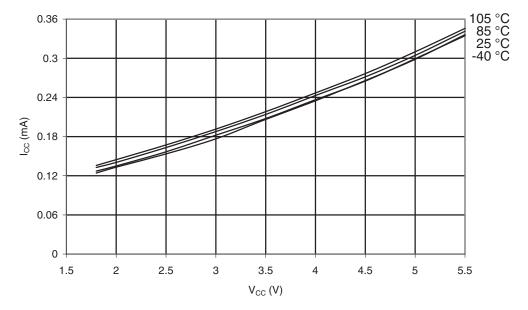
Figure 31-85. Idle Supply Current vs. V<sub>CC</sub> (Internal RC Oscillator, 1 MHz)
