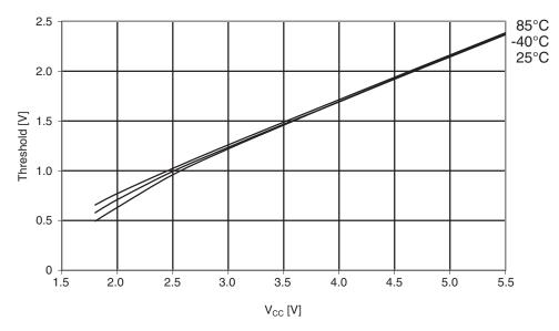
Figure 30-321. ATmega1284: I/O pin input threshold vs.  $V_{CC}$  ( $V_{IL}$ , I/O pin read as '0')
