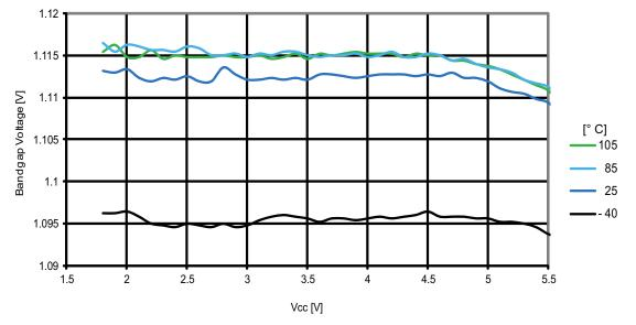
Figure 31-149. ATmega1284P: Calibrated bandgap voltage vs. V<sub>cc</sub>
