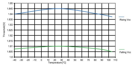
Figure 31-27. ATmega164PA: BOD threshold vs. temperature (V<sub>BOT</sub> = 1.8V)
