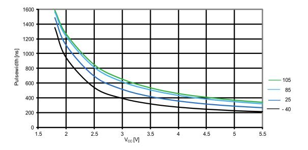
Figure 31-41. ATmega164PA: Minimum reset pulsewidth vs. V<sub>CC</sub>
