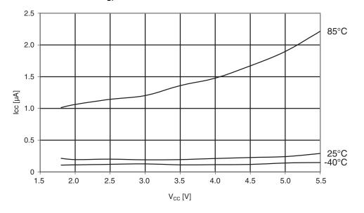
Figure 30-209. ATmega644A: Power-save supply current vs. V<sub>CC</sub> (watchdog timer disabled and 32kHz crystal oscillator running)
