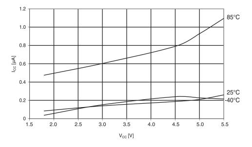
Figure 30-109. ATmega324A: Power-down supply current vs. V<sub>cc</sub> (watchdog timer disabled)
