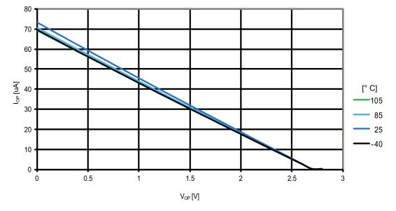
Figure 31-130. ATmega1284P: I/O pin pull-up resistor current vs. input voltage (V<sub>cc</sub> = 2.7V)
