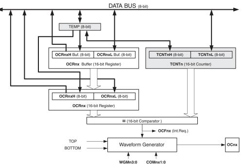
Figure 16-4. Output Compare unit, block diagram
