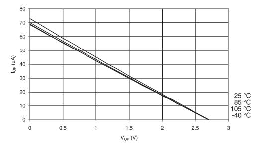
Figure 31-52. I/O Pin Pull-up Resistor Current vs. Input Voltage (V<sub>cc</sub> = 5V)
