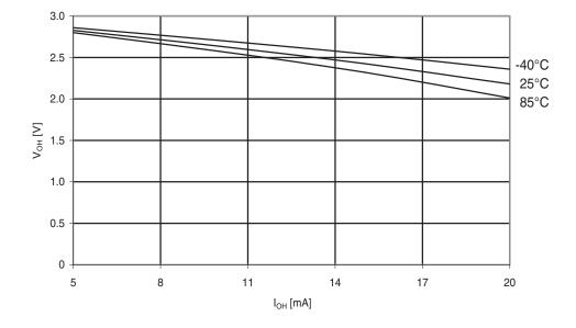
Figure 30-121. ATmega324A: I/O pin output voltage vs. source current (V<sub>cc</sub> = 3V)
