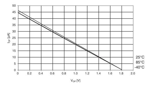
Figure 30-64. ATmega164PA: I/O pin pull-up resistor current vs. input voltage (V<sub>cc</sub> = 1.8V)
