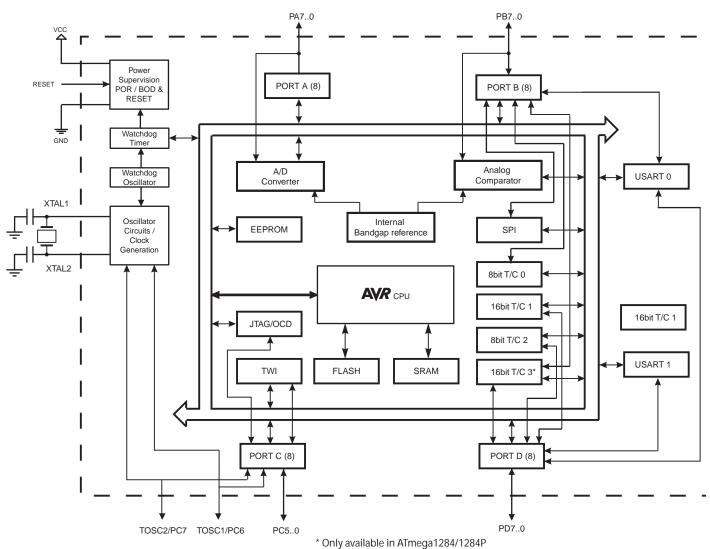
Figure 2-1. Block diagram
