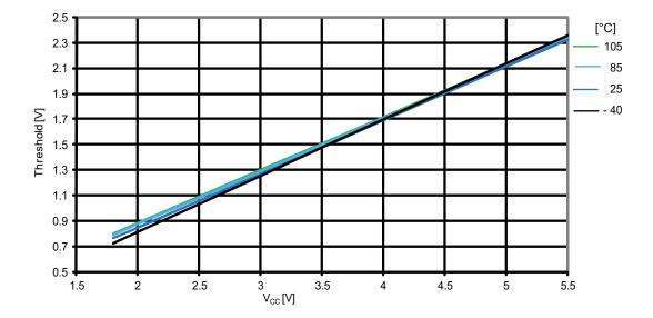
Figure 31-23. ATmega164PA: Reset pin input threshold vs. V<sub>CC</sub> (V<sub>IL</sub>, I/O pin read as '0')
