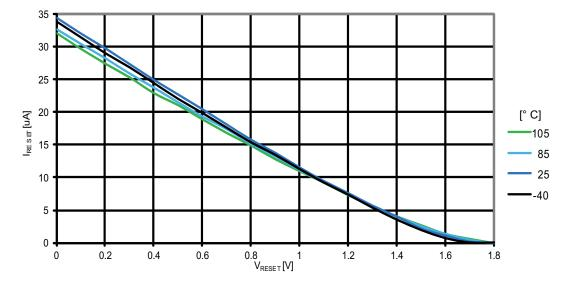
Figure 31-132. ATmega1284P: Reset pull-up resistor current vs. reset pin voltage (V<sub>cc</sub> = 1.8V)
