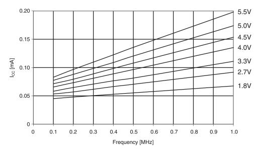
Figure 30-6. ATmega164A: Idle supply current vs. V<sub>CC</sub> (0.1 - 1.0MHz)
