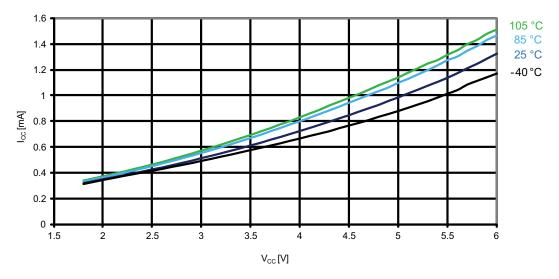
Figure 31-123. ATmega1284P: Idle supply current vs. V<sub>CC</sub> (internal RC oscillator, 8MHz)
