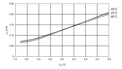
Figure 30-152. ATmega324PA: Active supply current vs. V<sub>cc</sub> (internal RC oscillator, 128kHz)
