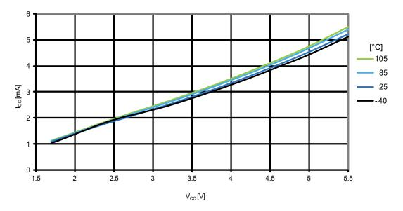
Figure 31-1. ATmega164PA: Active supply current vs. V<sub>CC</sub> (internal RC oscillator, 8MHz)
