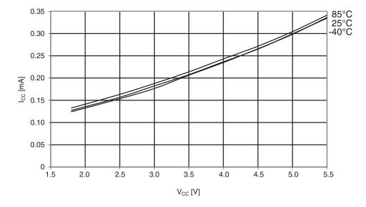
Figure 30-254. ATmega644PA: Idle supply current vs. V<sub>CC</sub> (internal RC oscillator, 1MHz)
