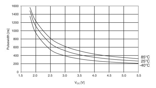
Figure 30-49. ATmega164A: Minimum reset pulsewidth vs. V<sub>cc</sub>
