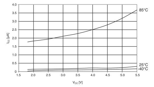
Figure 30-305. ATmega1284: Power-down supply current vs. V<sub>CC</sub> (watchdog timer disabled)
