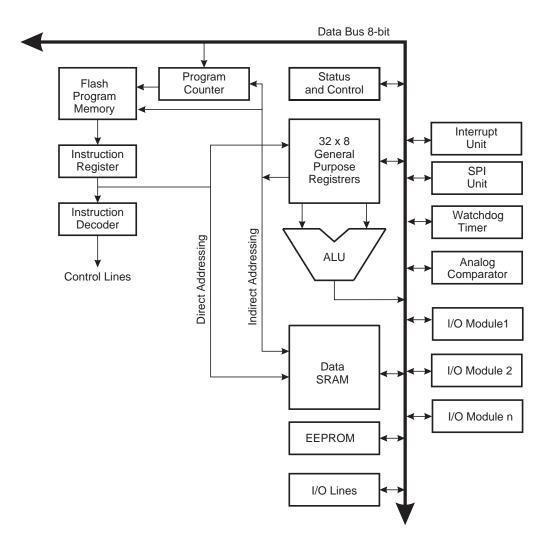
In order to maximize performance and parallelism, the AVR uses a Harvard architecture – with separate memories and buses for program and data. Instructions in the program memory are executed with a single level pipelining. While one instruction is being executed, the next instruction is pre-fetched from the program memory. This concept enables instructions to be executed in every clock cycle. The program memory is In-System Reprogrammable Flash memory.
