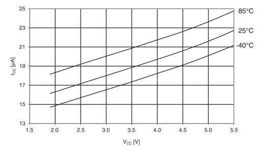
Figure 30-339. ATmega1284: Brownout detector current vs. V<sub>cc</sub>
