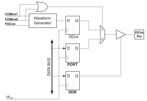
Figure 17-4. Compare Match Output unit, schematic
