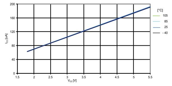
Figure 31-37. ATmega164PA: AREF external reference current vs. V<sub>cc</sub>
