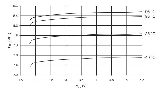
Figure 31-72. Calibrated 8 MHz RC Oscillator vs. Temperature
