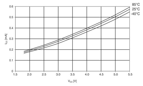
Figure 30-107. ATmega324A: Idle supply current vs. V<sub>cc</sub> (internal RC oscillator, 1MHz)
