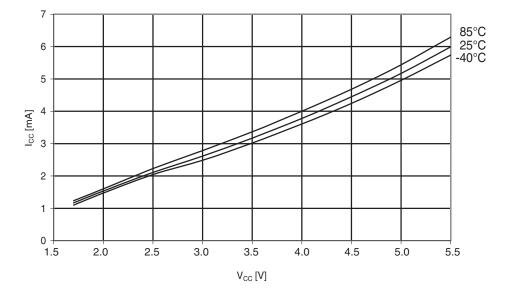
Figure 30-150. ATmega324PA: Active supply current vs. V<sub>CC</sub> (internal RC oscillator, 8MHz)
