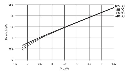
Figure 31-62. I/O Pin Input Hysteresis vs. V<sub>CC</sub>
