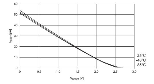
Figure 30-19. ATmega164A: Reset pull-up resistor current vs. reset pin voltage (V<sub>CC</sub> = 2.7V)
