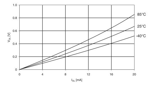
Figure 30-70. ATmega164PA: I/O pin output voltage vs. sink current (V<sub>CC</sub> = 3V)
