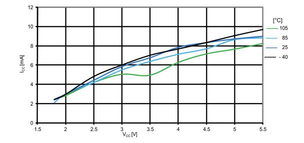
Figure 31-39. ATmega164PA: Programming current vs. V<sub>cc</sub>
