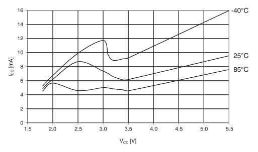
Figure 30-242. ATmega644A: Watchdog timer current vs. V<sub>CC</sub>
