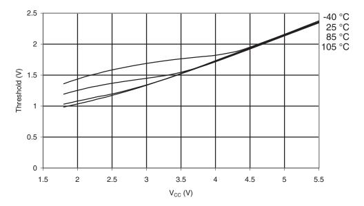
Figure 31-64. Reset Pin Input Threshold vs.  $V_{CC}$  (V<sub>IL</sub>, I/O Pin Read as '0')
