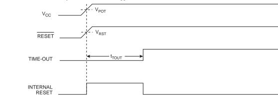
Figure 11-2. MCU Start-up, RESET Tied to V<sub>cc</sub>
