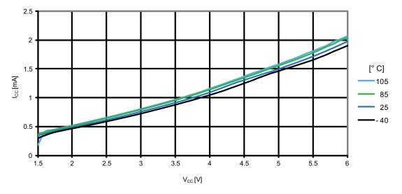
Figure 31-121. ATmega1284P: Active supply current vs. V<sub>CC</sub> (internal RC oscillator, 1MHz)
