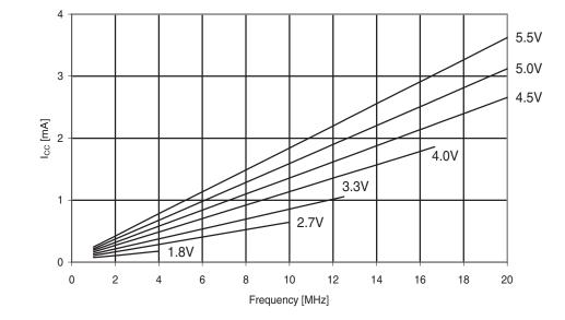
Figure 30-154. ATmega324PA: Idle supply current vs. V<sub>cc</sub> (1 - 20MHz)
