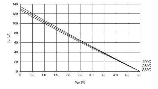
Figure 30-361. ATmega1284P: I/O pin pull-up resistor current vs. input voltage (V<sub>cc</sub> = 5V)
