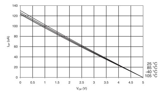
Figure 31-91. I/O Pin Pull-up Resistor Current vs. Input Voltage (V<sub>cc</sub> = 5V)
