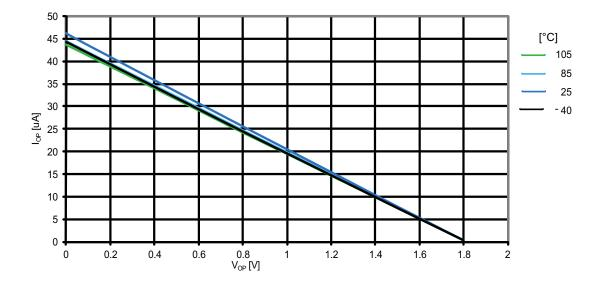
Figure 31-9. ATmega164PA: I/O pin pull-up resistor current vs. input voltage (V<sub>CC</sub> = 1.8V)
