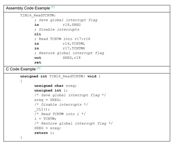
Note: 1. The example code assumes that the part specific header file is included. For I/O Registers located in extended I/O map, "IN", "OUT", "SBIS", "SBIC", "CBI", and "SBI" instructions must be replaced with instructions that allow access to extended I/O. Typically "LDS" and "STS" combined with "SBRS", "SBRC", "SBR", and "CBR".
