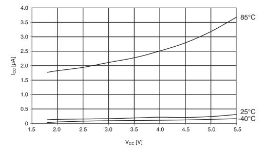
Figure 30-355. ATmega1284P: Power-down supply current vs. V<sub>CC</sub> (watchdog timer disabled)
