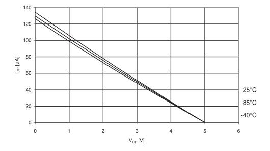
Figure 30-115. ATmega324A: I/O pin pull-up resistor current vs. input voltage (V<sub>cc</sub> = 5V)
