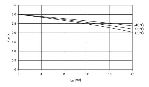
Figure 30-72. ATmega164PA: I/O pin output voltage vs. source current (V<sub>cc</sub> = 3V)
