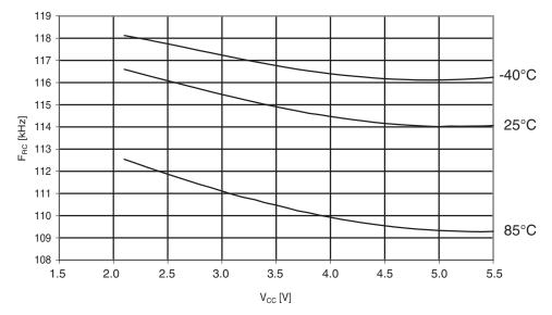
Figure 30-233. ATmega644A: Watchdog oscillator frequency vs. V<sub>cc</sub>
