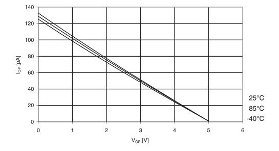
Figure 30-17. ATmega164A: I/O pin pull-up resistor current vs. input voltage (V<sub>cc</sub> = 5V)
