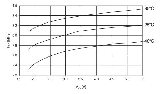
Figure 30-383. ATmega1284P: Calibrated 8MHz RC oscillator vs. V<sub>cc</sub>
