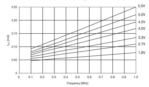
Figure 30-104. ATmega324A: Idle supply current vs. V<sub>cc</sub> (0.1 - 1.0MHz)
