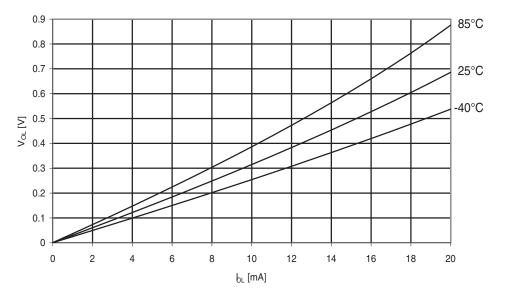
Figure 30-266. ATmega644PA: I/O pin output voltage vs. sink current (V<sub>CC</sub> = 3V)
