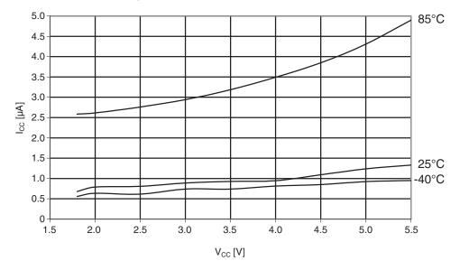
Figure 30-307. ATmega1284: Power-save supply current vs. V<sub>CC</sub> (watchdog timer disabled and 32kHz crystal oscillator running)
