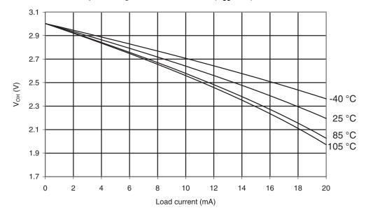
Figure 31-97. I/O Pin Output Voltage vs. Source Current (V<sub>cc</sub> = 3V)
