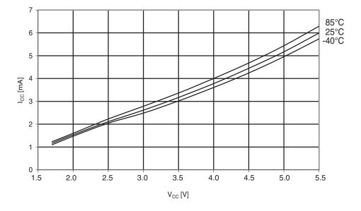
Figure 30-101. ATmega324A: Active supply current vs. V<sub>cc</sub> (internal RC oscillator, 8MHz)
