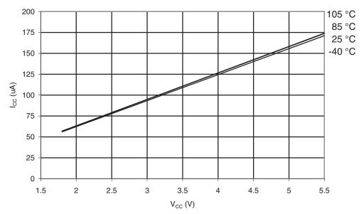
Figure 31-116. Brownout Detector Current vs. V<sub>cc</sub>
