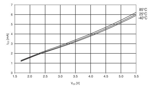
Figure 30-248. ATmega644PA: Active supply current vs. V<sub>cc</sub> (internal RC oscillator, 8MHz)
