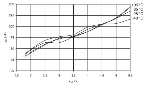
Figure 31-113. ADC Current vs. V<sub>CC</sub> (AREF = AV<sub>CC</sub>)
