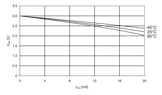
Figure 30-23. ATmega164A: I/O pin output voltage vs. source current (V<sub>cc</sub> = 3V)
