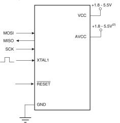
Notes: 1. If the device is clocked by the internal oscillator, it is no need to connect a clock source to the XTAL1 pin. 2.  $V_{CC} - 0.3V < AVCC < V_{CC} + 0.3V$ , however, AVCC should always be within 1.8 - 5.5V.
