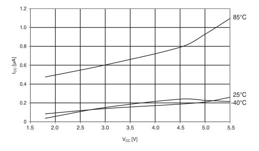
Figure 30-158. ATmega324PA: Power-down supply current vs. V<sub>CC</sub> (watchdog timer disabled)
