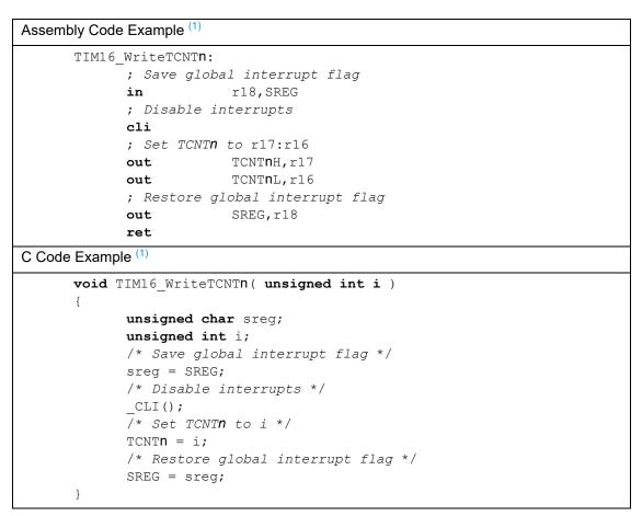
The example code assumes that the part specific header file is included. For I/O Registers located in extended I/O map, "IN", "OUT", "SBIS", "SBIC", "CBI", and "SBI" instructions must be replaced with instructions that allow access to extended I/O. Typically "LDS" and "STS" combined with "SBRS", "SBRC", "SBR", and "CBR".
