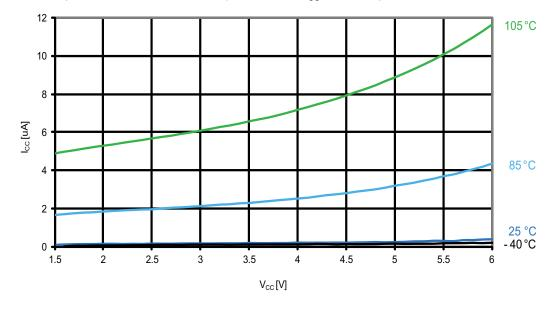
Figure 31-126. ATmega1284P: Power-down supply current vs. V<sub>cc</sub> (watchdog timer disabled)
