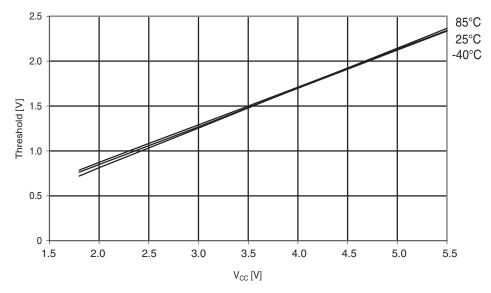
Figure 30-274. ATmega644PA: Reset pin input threshold vs. V<sub>CC</sub> (V<sub>IL</sub>, I/O pin read as '0')
