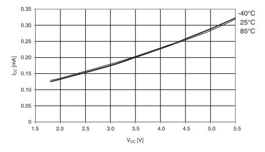
Figure 30-58. ATmega164PA: Idle supply current vs. V<sub>cc</sub> (internal RC oscillator, 1MHz)
