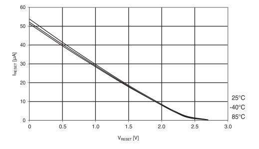
Figure 30-166. ATmega324PA: Reset pull-up resistor current vs. reset pin voltage (V<sub>cc</sub> = 2.7V)
