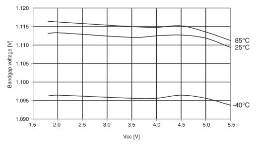
Figure 30-379. ATmega1284P: Calibrated bandgap voltage vs. V<sub>cc</sub>
