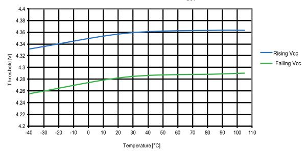
Figure 31-146. ATmega1284P: BOD threshold vs. temperature (V<sub>BOT</sub> = 4.3V)
