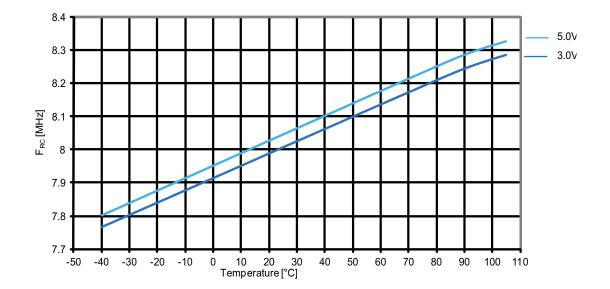
Figure 31-33. ATmega164PA: Calibrated 8MHz RC oscillator vs. temperature
