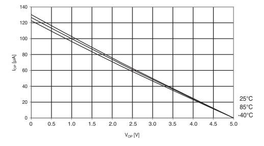
Figure 30-213. ATmega644A: I/O pin pull-up resistor current vs. input voltage (V<sub>cc</sub> = 5V)
