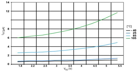
Figure 31-128. ATmega1284P: Power-save supply current vs. V<sub>CC</sub> (watchdog timer disabled and 32kHz crystal oscillator running)
