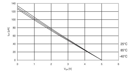
Figure 30-164. ATmega324PA: I/O pin pull-up resistor current vs. input voltage (V<sub>cc</sub> = 5V)
