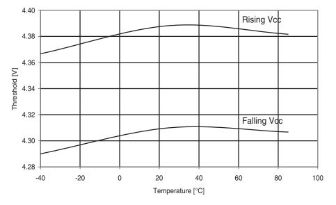
Figure 30-129. ATmega324A: BOD threshold vs. temperature (V<sub>BOT</sub> = 4.3V)
