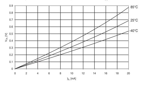
Figure 30-217. ATmega644A: I/O pin output voltage vs. sink current (V<sub>cc</sub> = 3V)
