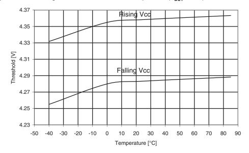
Figure 30-326. ATmega1284: BOD threshold vs. temperature (V<sub>BOT</sub> = 4.3V)
