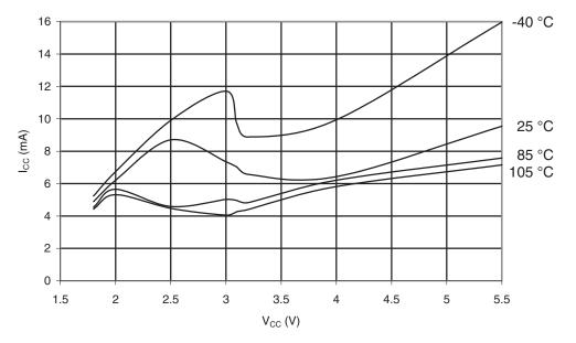
Figure 31-118. Watchdog Timer Current vs. V<sub>cc</sub>
