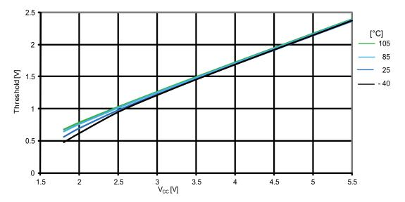
Figure 31-21. ATmega164PA: I/O pin input hysteresis vs. V<sub>cc</sub>
