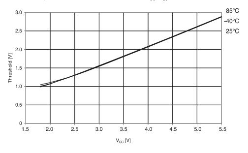
Figure 30-172. ATmega324PA: I/O pin input threshold vs. V<sub>CC</sub> (V<sub>IH</sub> , I/O pin read as '1')
