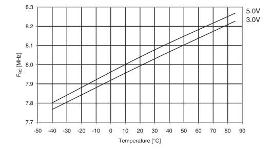
Figure 30-88. ATmega164PA: Calibrated 8MHz RC oscillator vs. temperature
