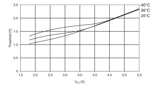
Figure 30-373. ATmega1284P: Reset pin input threshold vs. V<sub>CC</sub> (V<sub>IH</sub> , I/O pin read as '1')
