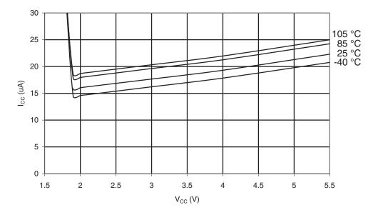
Figure 31-78. Programming Current vs. V<sub>CC</sub>
