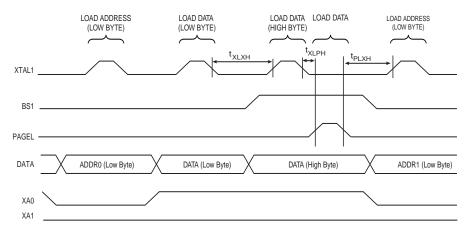
Note: 1. The timing requirements shown in Figure 27-7 (that is,  $t_{DVXH}$ ,  $t_{XHXL}$ , and  $t_{XLDX}$ ) also apply to loading operation.
