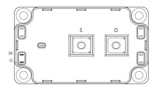
$V_{DSS} = 1200V$   $R_{DSon} = 100m\Omega \text{ typ } @ \text{Tj} = 25^{\circ}\text{C}$   $I_D = 116A @ \text{Tc} = 25^{\circ}\text{C}$
