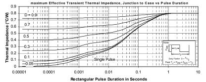
Typical SiC parallel diode Performance Curve
