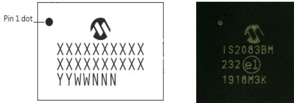
Figure 9-4. IS2083BM Package Marking Information
