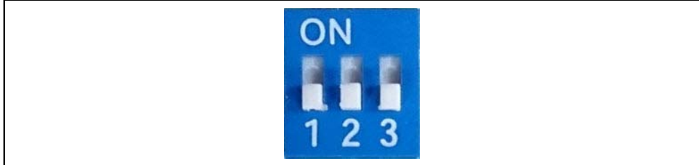
FIGURE 3-1: SW9 IN FLASH APPLICATION MODE
