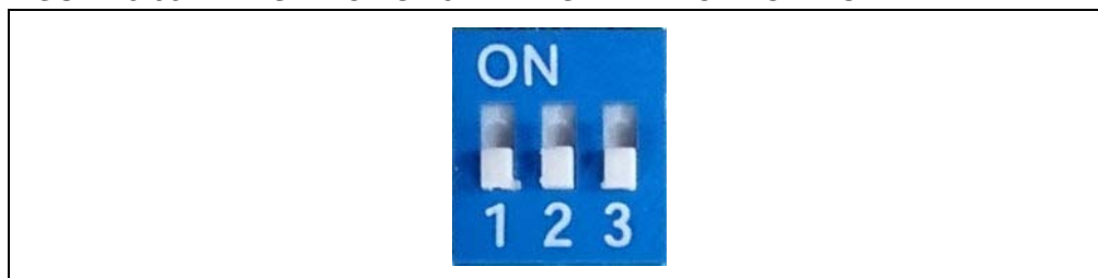
FIGURE 3-35: SWITCH SW9 IN FLASH APPLICATION MODE
