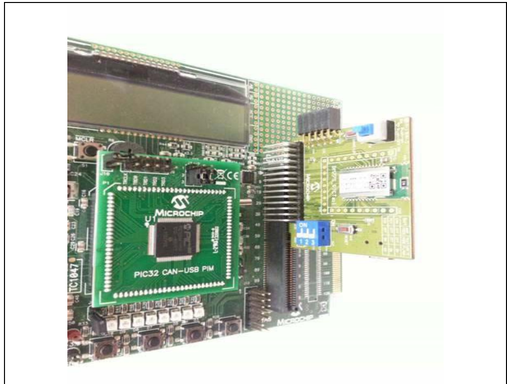
FIGURE 1-3: BM78 EVB BOARD INSERTED INTO PICtail™ INTERFACE
