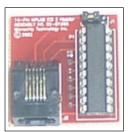
For 8-pin (PIC12F629/675), 14-pin (PIC16F630/676) or 18-pin (PIC16F627A/628A/648A) devices, limited I/O make integrated in-circuit debugging impractical. Instead, incircuit debugging is made possible by using a header containing an equivalent device with integrated incircuit debugging peripheral. For debugging, the header is connected
