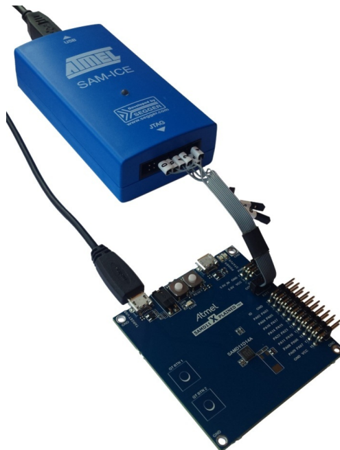
Figure 6-6. SAM-ICE using a Squid Cable
