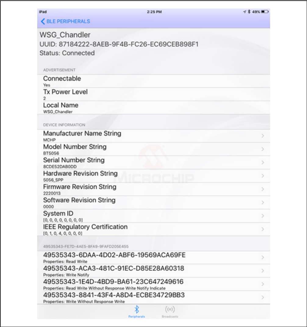
FIGURE 3-6: SMARTDISCOVER APP DISPLAYING THE GATT SERVICES AVAILABLE ON THE RN4678 MODULE
