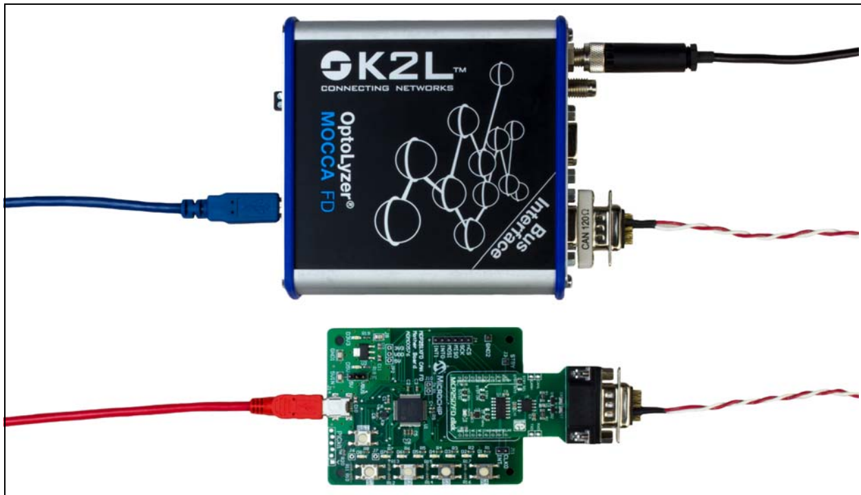
FIGURE 2-2: Connecting the MCP251XFD CAN FD Motherboard.
