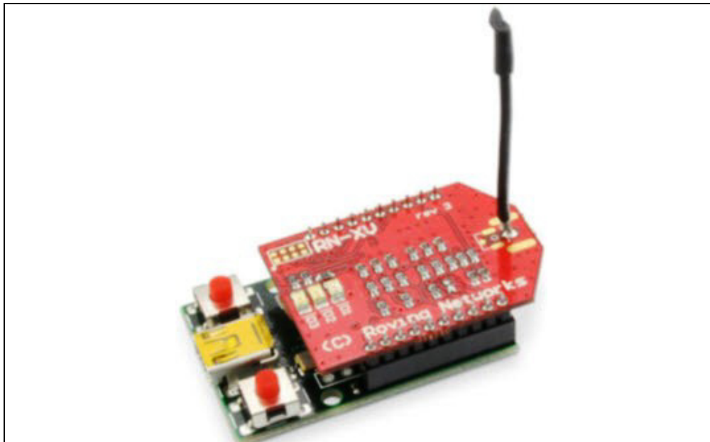
FIGURE 2-1: HARDWARE SETUP WITH RN171XV BOARD
