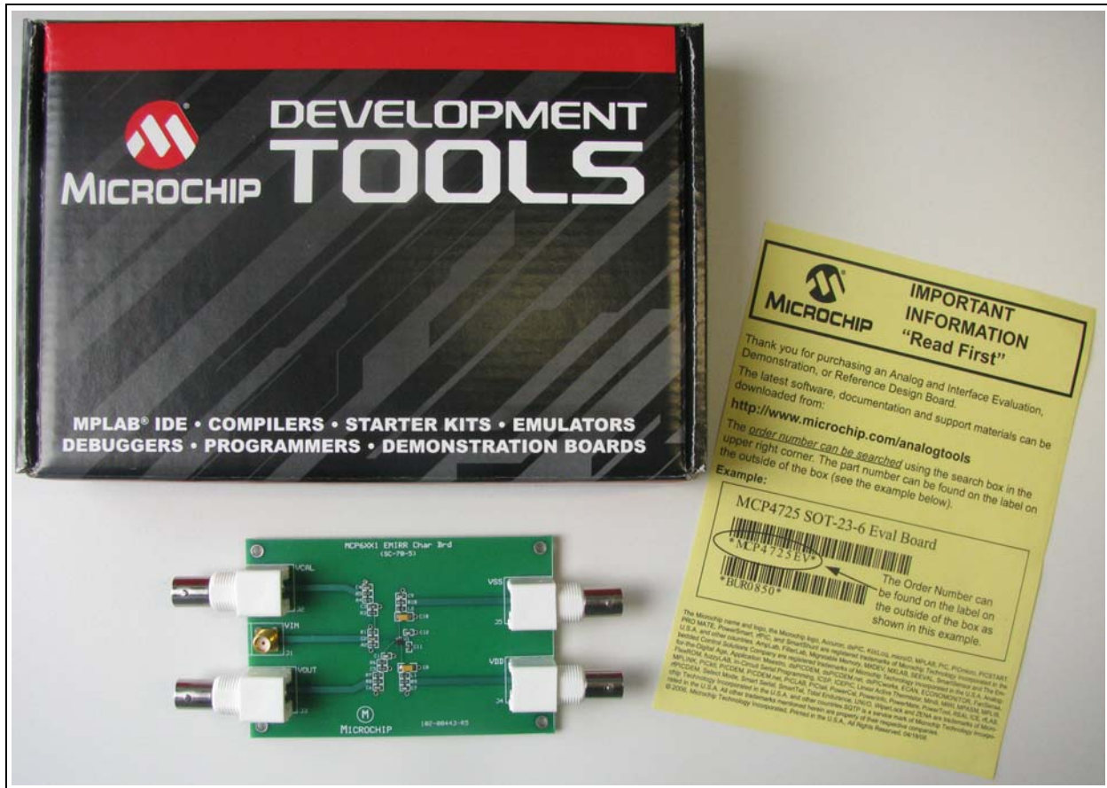
FIGURE 1-2: MCP6421 EMIRR Evaluation Board.
