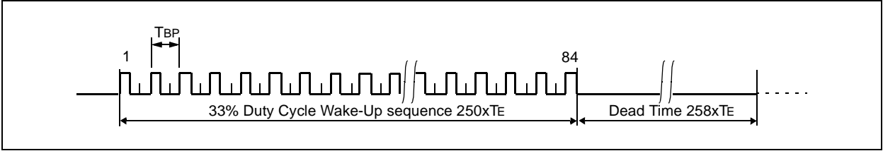
FIGURE 8-6: VPWM WAKE-UP FORMAT (MOD=1)
