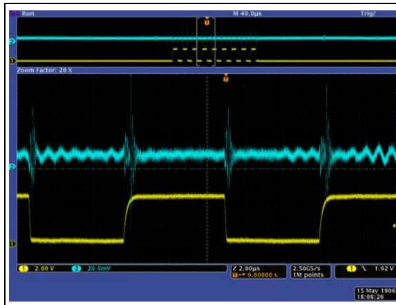
FIGURE 2-40: Digital Feedthrough (SCL signal coupling to V_{OUT} pin); V_{DD} = 5.0\text{V} , V_{REF} = 5.0\text{V} , F_{SCL} = 100\text{ kHz} , V_{OUT} = 20h ( V_{OUT} Voltage Scale = 20\text{ mV/div} , Time scale = 2\text{ }\mu\text{s / div} ).
