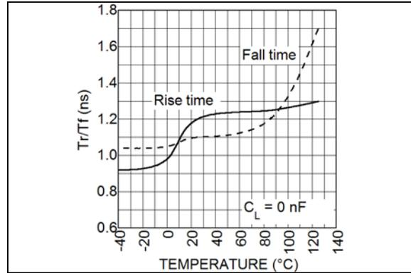
**FIGURE 2-11:** Rise and Fall Time (5V) vs. Temperature.
