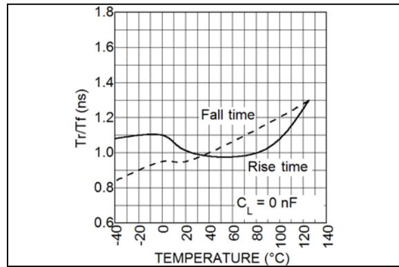
**FIGURE 2-12:** Rise and Fall Time (12V) vs. Temperature.
