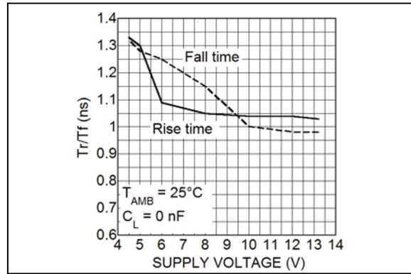
**FIGURE 2-10:** Rise and Fall Time vs. Supply Voltage.
