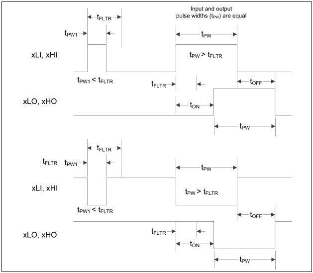
FIGURE 4-3: Minimum Pulse-Width Diagram.
