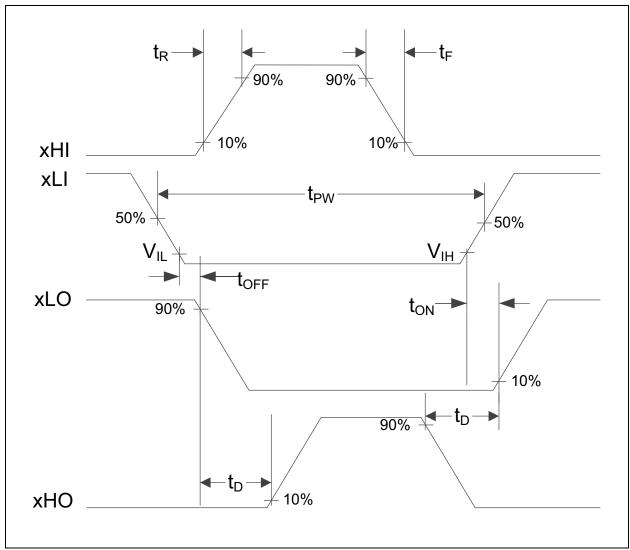
FIGURE 4-4: Dead Time, Propagation Delay, and Rise/Fall-Time Diagram.
