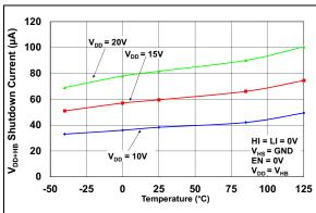
**FIGURE 2-8:** V<sub>DD+HB</sub> Shutdown Current vs. Temperature.
