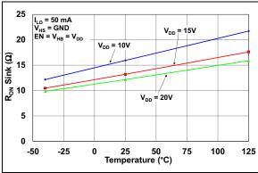
FIGURE 2-14: LO Output Sink ON-Resistance vs. Temperature.
