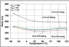
FIGURE 2-21: Propagation Delay vs. Temperature.
