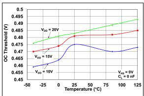
**FIGURE 2-32:** Overcurrent Threshold vs. Temperature.
