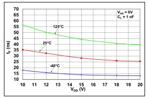
**FIGURE 2-25:** LO Fall Time vs.  $V_{DD}$  Voltage.
