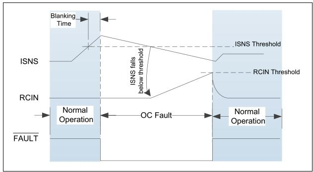
FIGURE 4-8: Overcurrent Fault Sequence.
