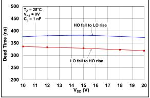
FIGURE 2-28: Dead Time vs. V<sub>DD</sub> Voltage.
