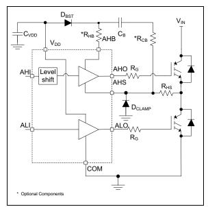
FIGURE 5-1: MIC4609 – Bootstrap Circuit.
