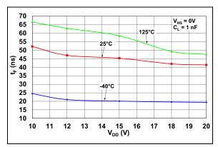
**FIGURE 2-23:** HO Fall Time vs.  $V_{DD}$  Voltage.
