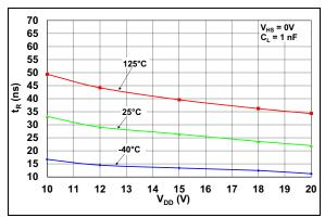
**FIGURE 2-24:** LO Rise Time vs.  $V_{DD}$  Voltage.
