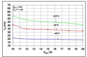
**FIGURE 2-22:** HO Rise Time vs.  $V_{DD}$  Voltage.
