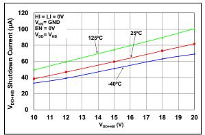
**FIGURE 2-7:** V<sub>DD+HB</sub> Shutdown Current vs. Voltage.
