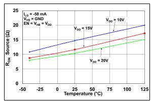
FIGURE 2-18: LO Output Source ON-Resistance vs. Temperature.
