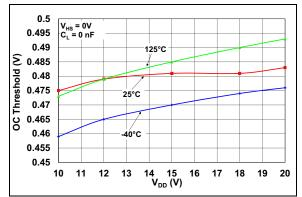
**FIGURE 2-31:** Overcurrent Threshold vs.  $V_{DD}$  Voltage.
