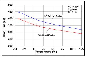
**FIGURE 2-29:** Dead Time vs. Temperature  $(V_{DD} = 10V)$ .
