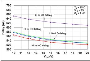
**FIGURE 2-20:** Propagation Delay vs.  $V_{DD}$  Voltage.
