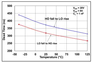
**FIGURE 2-30:** Dead Time vs. Temperature  $(V_{DD} = 20V)$ .
