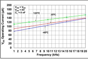
**FIGURE 2-9:**  $V_{DD}$  Operating Current vs. Frequency.
