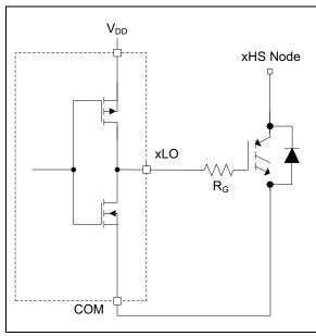
FIGURE 4-5: Low-Side Driver Block Diagram.
