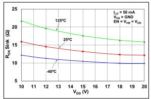
**FIGURE 2-13:** LO Output Sink ON-Resistance vs.  $V_{DD}$ .
