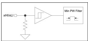
FIGURE 4-2: Input Stage Block Diagram.
