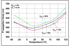
**FIGURE 2-34:** Overcurrent Propagation Delay vs. Temperature.
