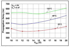
**FIGURE 2-33:** Overcurrent Propagation Delay vs. V<sub>DD</sub> Voltage.
