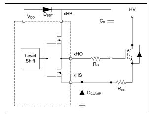
FIGURE 4-6: High-Side Driver and Bootstrap Circuit Block Diagram.
