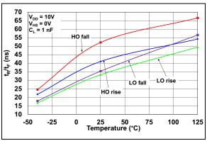
**FIGURE 2-26:** Rise/Fall Time vs. Temperature  $(V_{DD} = 10V)$ .
