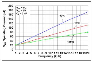
**FIGURE 2-10:** V<sub>HB</sub> Operating Current vs. Frequency – One Phase.
