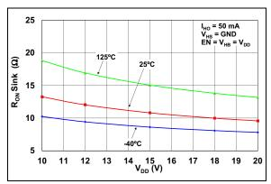
**FIGURE 2-11:** HO Output Sink ON-Resistance vs.  $V_{DD}$ .
