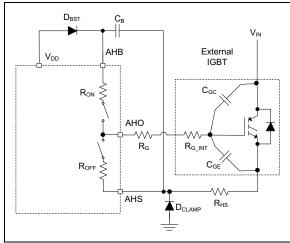
**FIGURE 5-3:** MIC4609 High-Side Driving an External IGBT.
