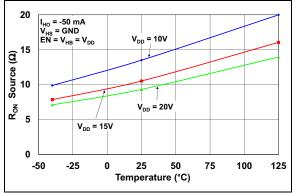
FIGURE 2-16: HO Output Source ON-Resistance vs. Temperature.
