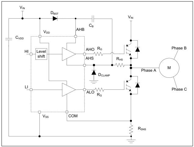
FIGURE 4-7: MIC4609 Motor Driver Typical Application – Phase A.
