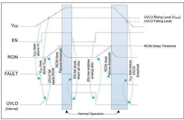
FIGURE 4-1: Startup and Fault Timing Diagram.
