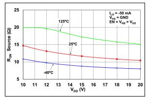
**FIGURE 2-17:** LO Output Source ON-Resistance vs.  $V_{DD}$ .
