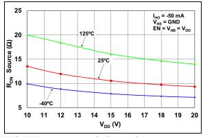
**FIGURE 2-15:** HO Output Source ON-Resistance vs.  $V_{DD}$ .
