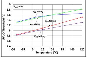
**FIGURE 2-19:**  $V_{DD}/V_{HB}$  ULVO vs. Temperature.
