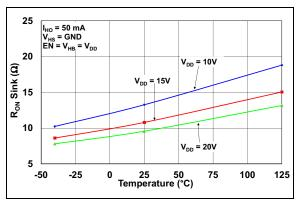
**FIGURE 2-12:** HO Output Sink ON-Resistance vs. Temperature.
