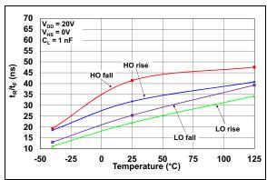
**FIGURE 2-27:** Rise/Fall Time vs. Temperature ( $V_{DD} = 20V$ ).
