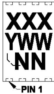
8-Lead TDFN (2x3x0.75 mm) ( MCP6V62 )
