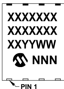
8-Lead DFN-S (6x5x0.9 mm)
