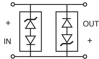
Optional Bidirectional configuration (two TVS devices in parallel)
