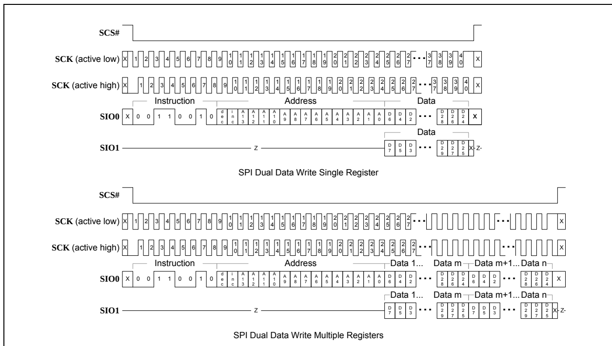
FIGURE 10-13: SPI DUAL DATA WRITE
