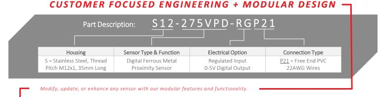
HOUSING - Aluminum, stainless steel, plastic, threaded, flange mount, customer specific
