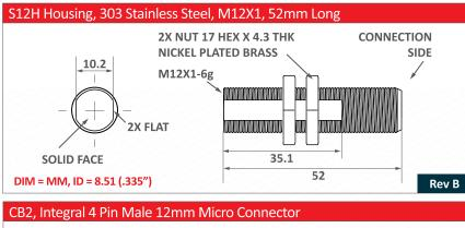
12MM X 1 THREADS (PART OF HOUSING) **SENSOR** HOUSING SENSOR BACK VIEW SHOWING PINS ADDS 1MM TO HOUSING LENGTH Rev A
