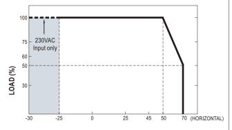
AMBIENT TEMPERATURE WITH 128 CFM FAN\*2 OR WATER COOLING SYSTEM ( $^{\circ}\text{C}$  )
