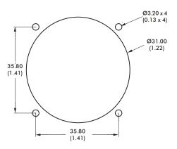
The joystick is mounted beneath the panel and the base of the bootmust be brought through the panel cut-out and held in place with the circular bezel. For panel thickness of <3mm, M3 x 16 countersunk machine screws are recommended.
