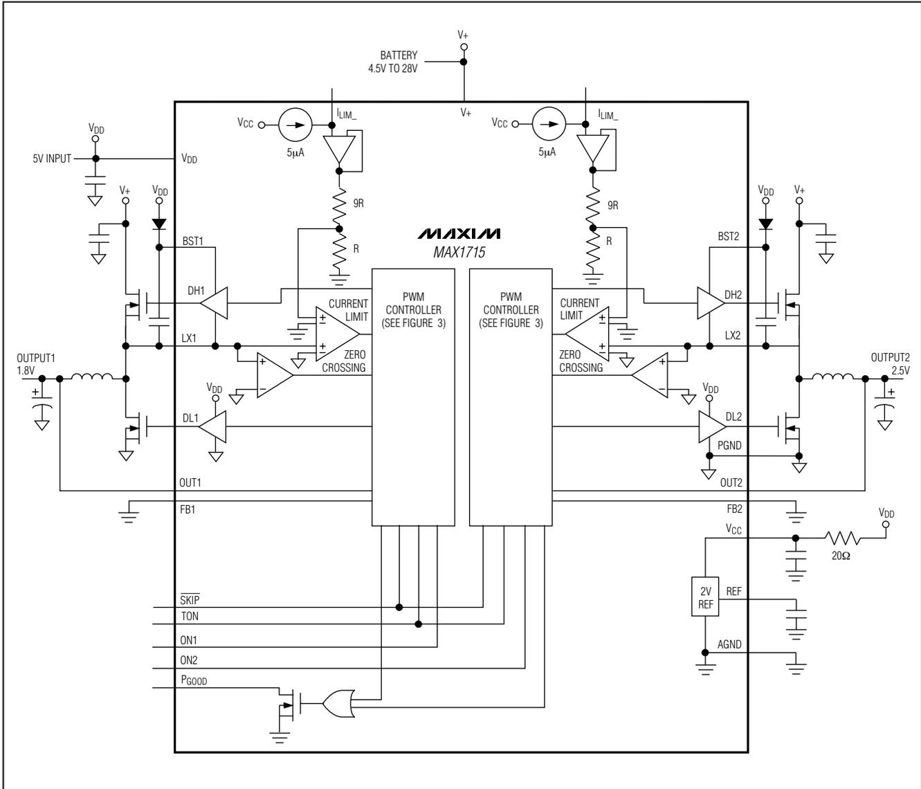
Figure 2. Functional Diagram
