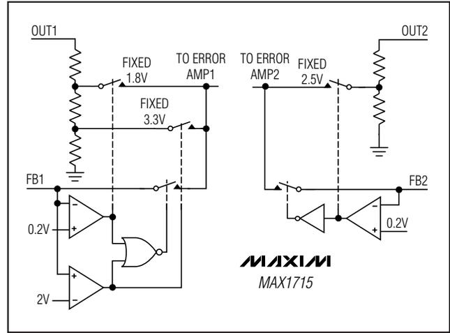
Figure 9. Feedback Mux
