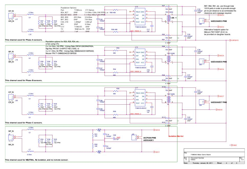
Figure 4-3: Teridian 71M6543 REV 4.0 Demo Board: Electrical Schematic 3/4
