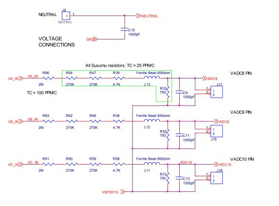
If high-precision Rs are not available, use: Vishay P/N RN65D2004FB14 Mouser P/N 71-RN65D-F-2.0M TC = 100 PPM/C
