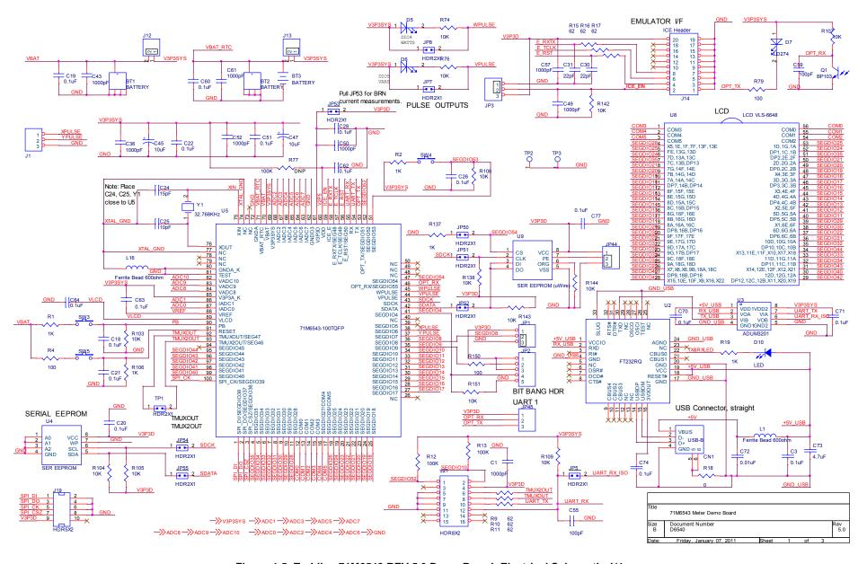
Figure 4-5: Teridian 71M6543 REV 5.0 Demo Board: Electrical Schematic 1/4
