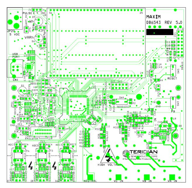
Figure 4-14: Teridian 71M6543 REV 5.0 Demo Board: Top View
