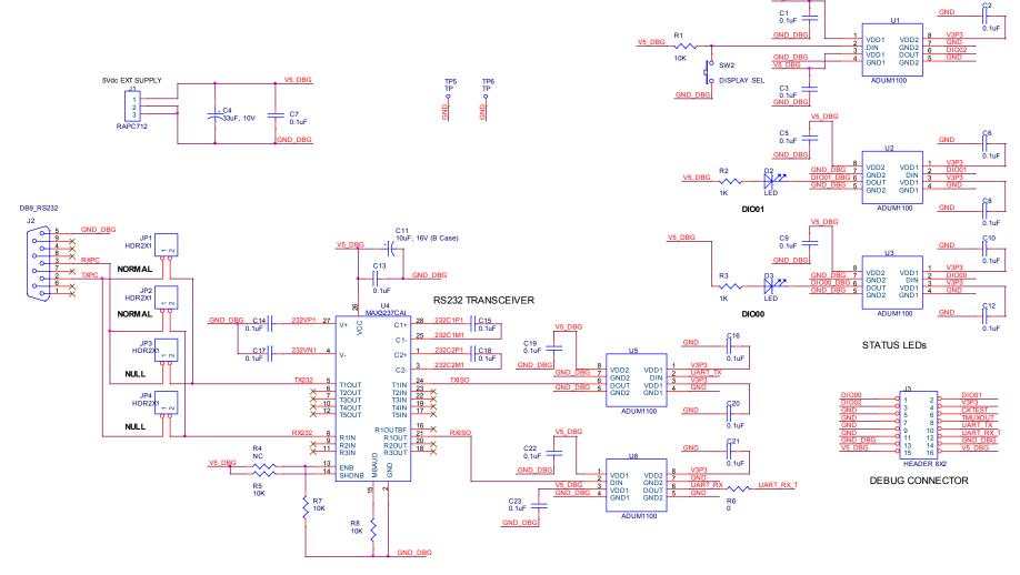
Figure 4-18: Debug Board: Electrical Schematic
