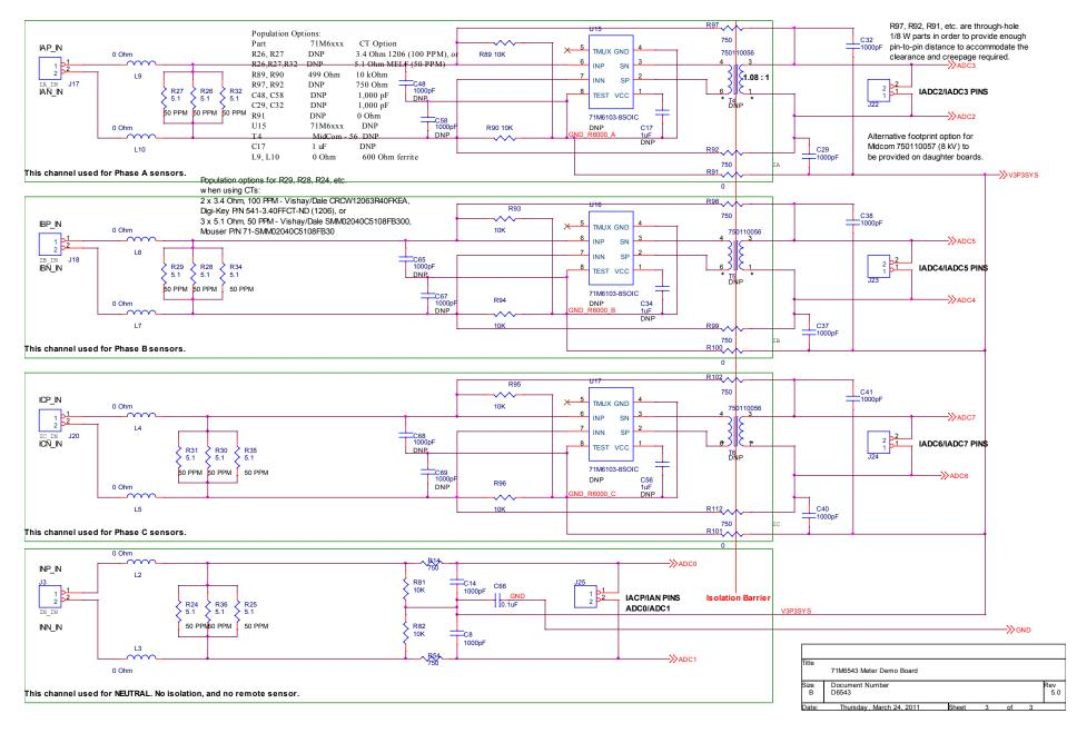
Figure 4-7: Teridian 71M6543 REV 5.0 Demo Board: Electrical Schematic 3/4
