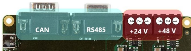
Figure 3: Power; Communication and USB-C connectors of TMCM-BB4
