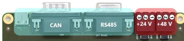
Figure 3: Power; Communication and USB-C connectors of TMCM-BB1
