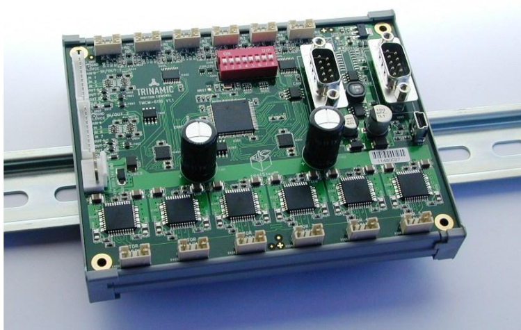
Figure 3.2 DIN rail mounting
