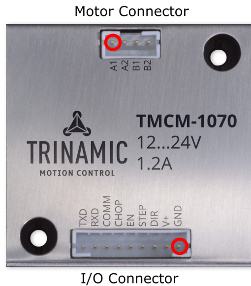
Figure 7: TMC-1070 connectors (pin 1 highlighted in red)
