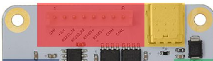
Figure 3: Power / communication connector of TMCM-0960-MotionPy V21
