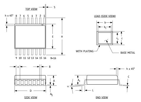
Figure 15.1 Dimensional drawings SSOP16, 150 MILS, 0.635mm (0.025 inch) pitch
