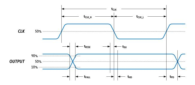
Figure 13.1 General timing parameters
